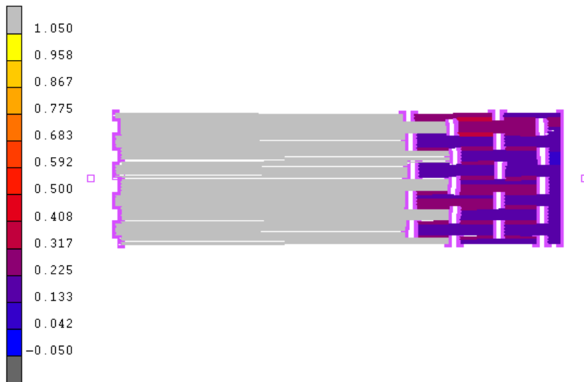
Figure 9.21. Distribution of strains for fibres in model at fabric strain of 1 (model FL-I but most fibres are located on right-hand side)
