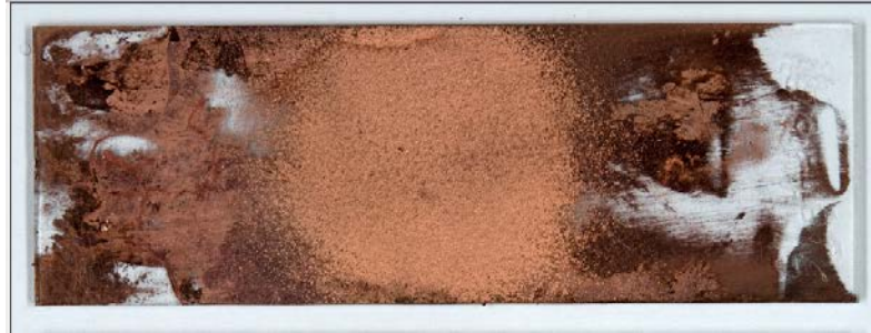
Figure 4.5 Electroless copper plating on roughened CMG glass without APTS pretreatment
