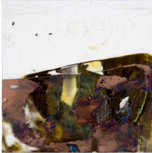
Figure 4.15 Oxidation of the copper coating on CMG glass
