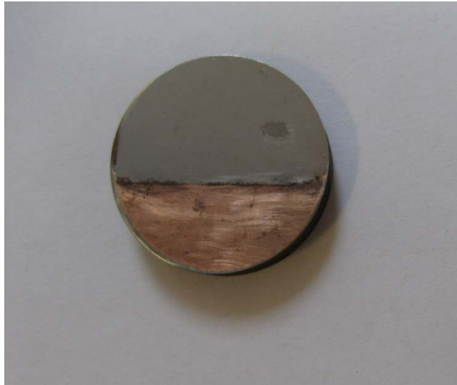
Figure 4.10 Copper coating step on steel coin sample
