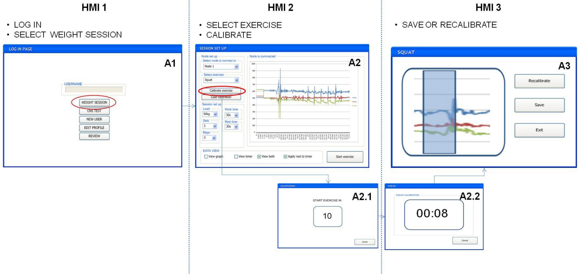
Figure 8.20 Software prototype: the HMI screen navigation designed to set up for a weights session.
