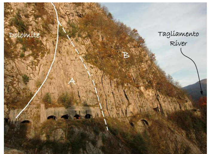
Figure 2. Limestone rock mass, Zone A is described as a compact rock mass while Zone B is characterized by open bedding discontinuities. The dashed line marks the boundary between Zones A and B and coincides with a poor Rock Quality Design (RQD <25%) band, two metres wide.
