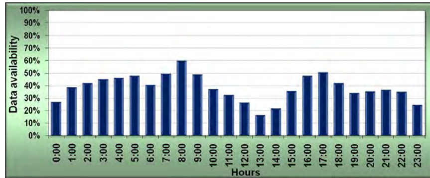
Figure 10. SST data available from GEOS Satellite during the day averaged over the entire study period between 25/07/2007 and 26/06/2009.
