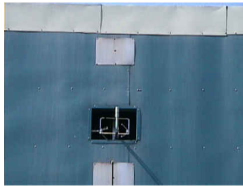
Figure 5. An ultrasonic anemometer, a static pressure probe placed at the high level opening and two pressure taps near the opening
