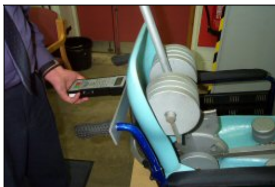
Figure 3: Measurement of push effort
