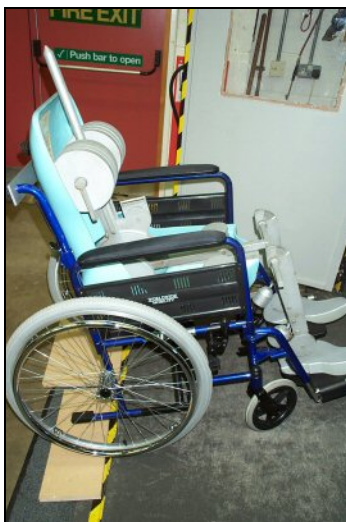
Figure 2: Wheelchair and manikin used in test measurements
