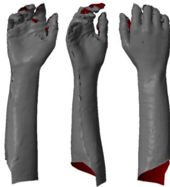
Figure 1(a): Polygonal mesh from direct 3D laser scanning
