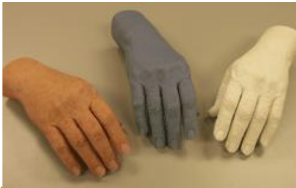
Figure 2: Prosthetic hand production. 3D scan data was captured by scanning a plaster cast (right), and was used to produce a realistic artificial hand fabricated by additive manufacture (left). Image courtesy of Direct Dimensions (2010)
