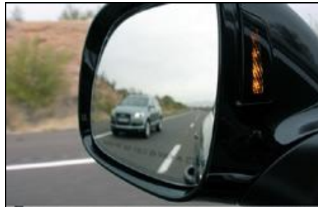
Figure 36: Audi side assist system – external mirror with LED warning http://www.autoblog.com/2006/03/21/video-animation-of-audi-s-trick-side-assist/
