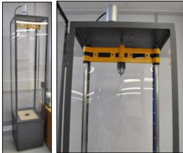
Figure 2 : In-house manufactured impact rig to HOSDB requirements.
