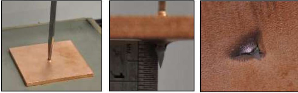
Figure 6 : 4.5mm thick nanocrystalline copper metallised sample
