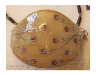
The effective local force can be calculated by using the measured pressure and the area
