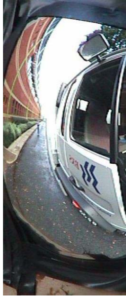
Figure 68. Foreshortening of vehicle's length through 200mm roc mirror
