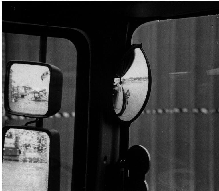
Figure 23. Internally mounted, small radius of curvature mirror viewing immediate frontal area of an HGV.
