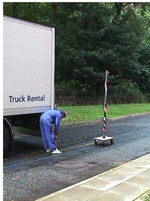
Figure 64. Measuring reversing error using a simulated reversing task
