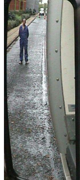
Figure 69. Foreshortening of vehicle's length through 200mm roc mirror
