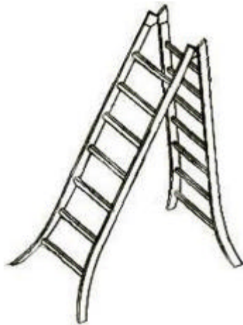
C. Standing rung ladder with splayed stiles
