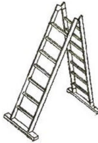
D. Standing rung ladder with parallel stiles and stabilisers
