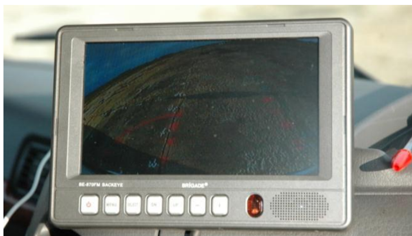
Figure 589. Internal screen of the camera system with the sun light shining onto the screen
