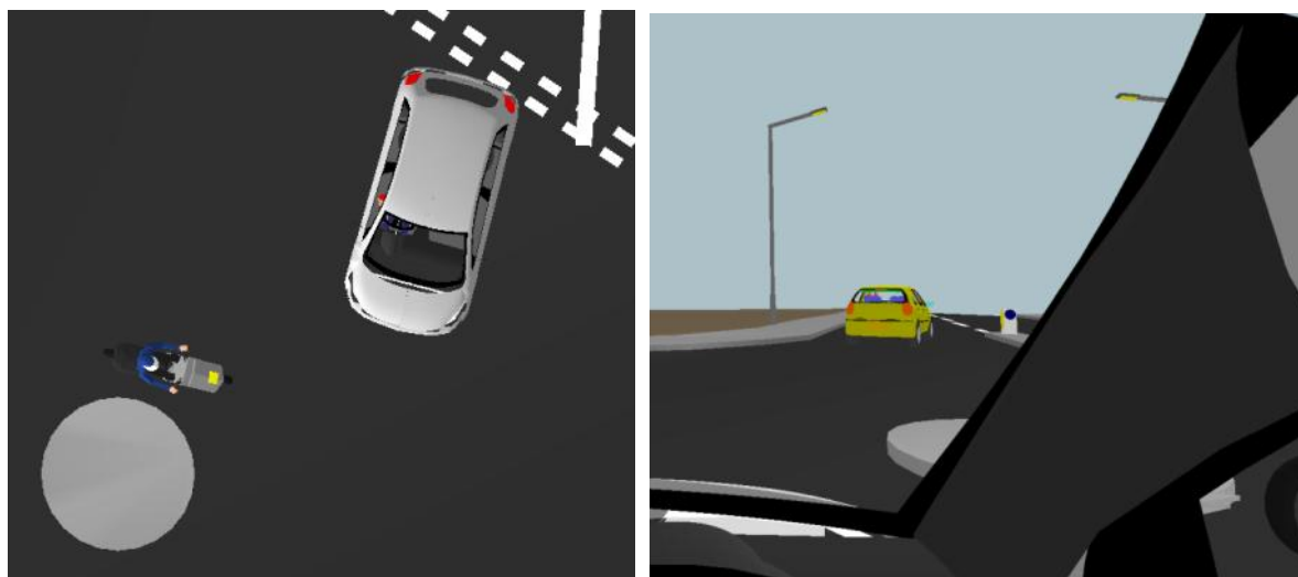
Figure 307. The scooter can effectively travel the whole distance until the point of impact obscured by the M_1 A-pillar
