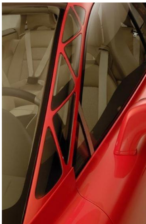
Figure 422. The webbed A-pillar of the Volvo SCC (courtesy of volvocars.com)
