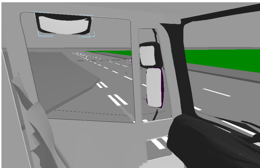
Figure 132. The driver's eye view: The approaching vehicle being partially obscured from the category N 2 Driver's vision due to the Class II and Class IV mirror surrounds
