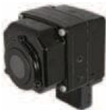
Figure 163. Brigade PathFindIR Thermal Imaging Camera
