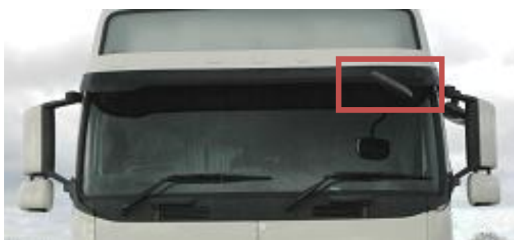
Figure 549. Class VI mounted in lateral position (Mirror within red box)
