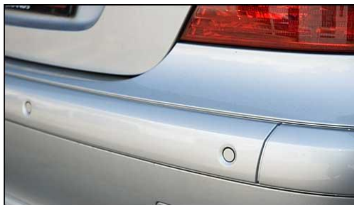
Figure 170. Typical Ultrasonic Reversing Sensor Installation on M 1 Vehicle
