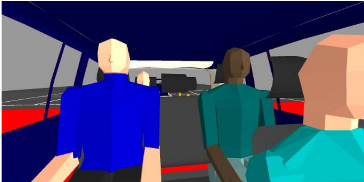
Figure 521. 1m Rearwards visibility with occupants (head restraints at highest setting)
