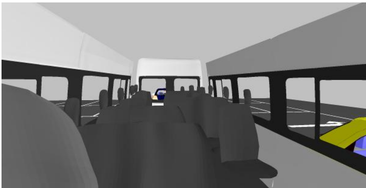
Figure 442. 1.47m Stature person (1%ile UK Female) rearwards of the vehicle (head restraints removed)
