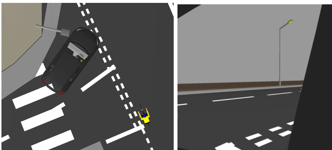
Figure 320. The cyclist can get within 4.5m of the M 1 whilst obscured by the B-pillar
