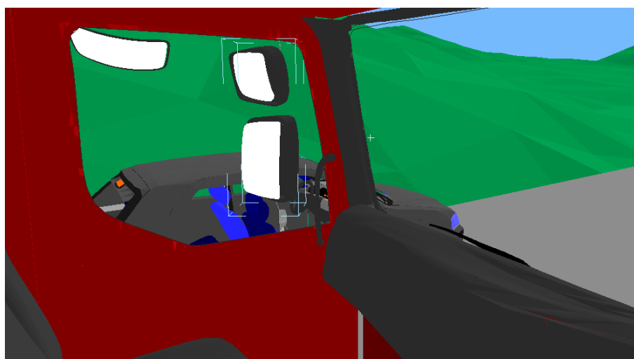
Figure 138. A car to the left of the driver's cab, and forward of the volume of space covered by the Class IV mirror is directly visible to a 99 th ile stature LGV driver
