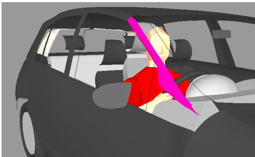
Figure 420. The size of A-pillar required to accommodate the 5%ile UK female in an inter-ocular solution
