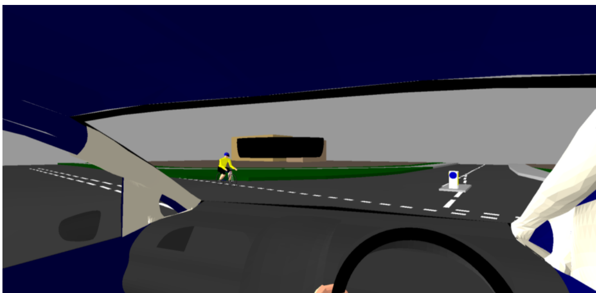
Figure 374. The cyclist needs to be a relatively long way to the left of the M 1 vehicle to stay hidden behind the A-pillar
