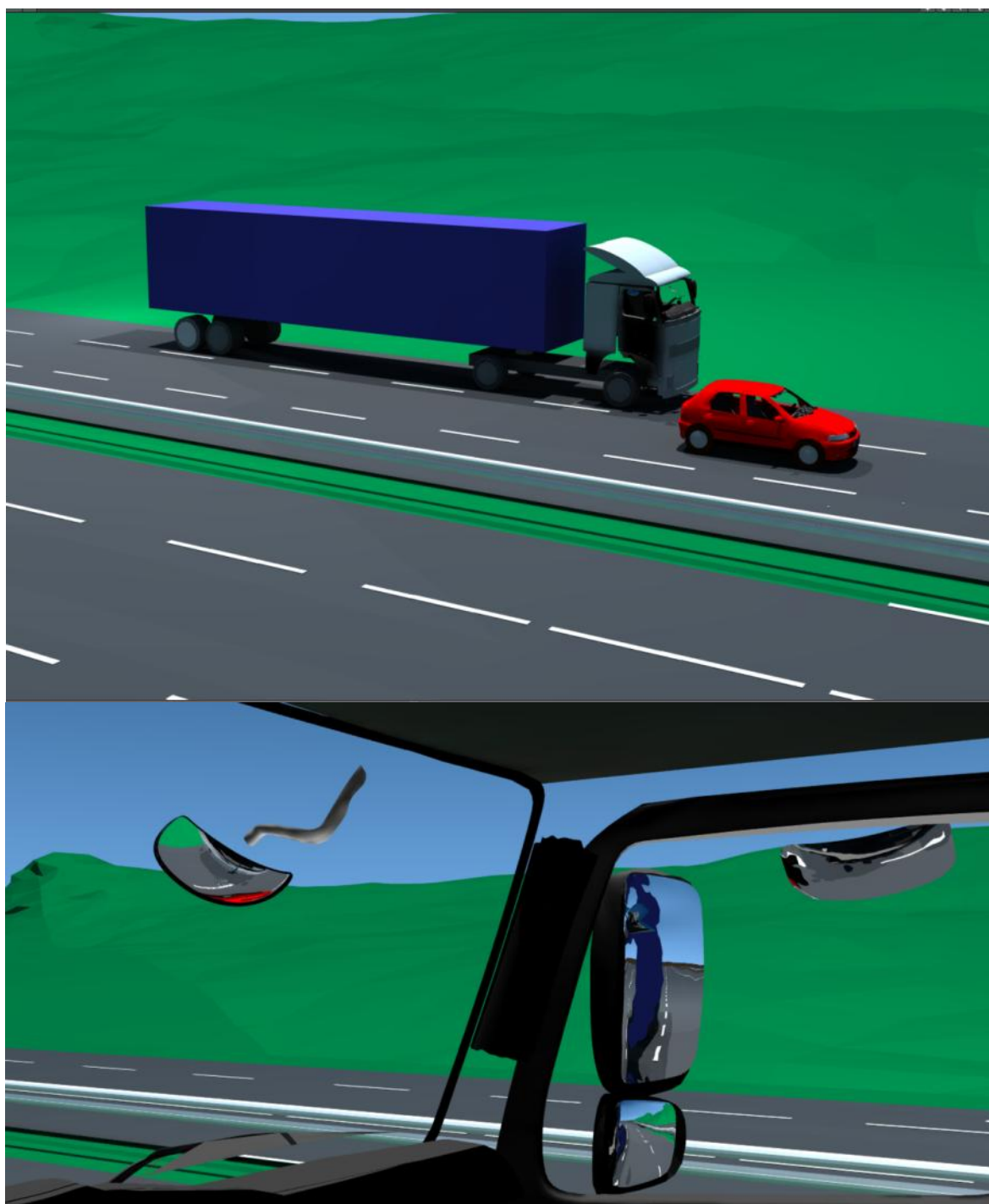
Figure 160. Stage 6: The vehicle is partially visible in the Class VI mirror
