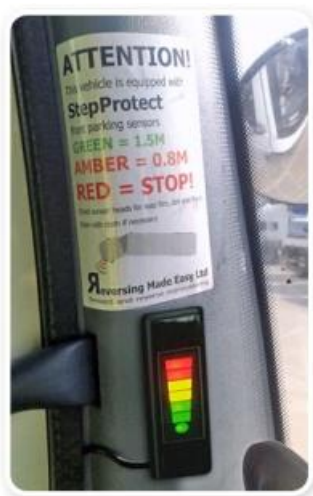
Figure 166. Example of Visual Warning System Mounted on the Nearside A-Pillar
