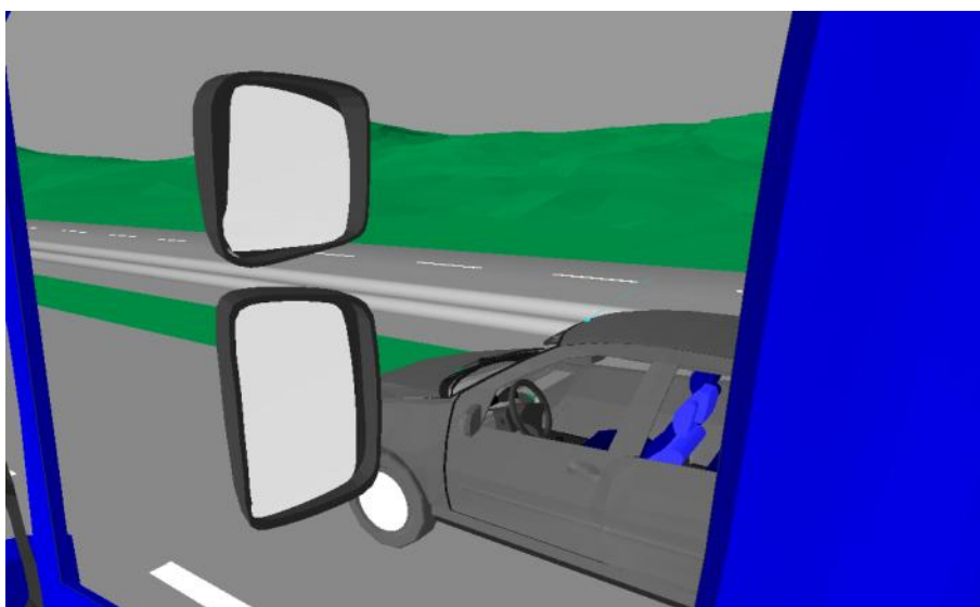
Figure 148. A car to the right of the driver's cab, and forward of the volume of space covered by the Class IV mirror is directly visible to a 4 th ile stature LGV driver
