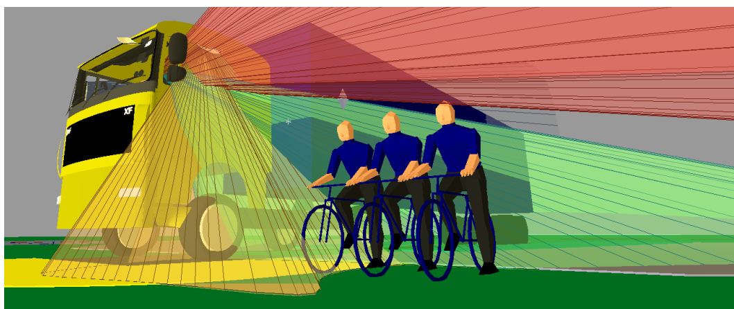
Figure 54. The blind spot between the Class V mirror and the volume that represents the direct vision through the passenger window for 99th%ile driver projections
