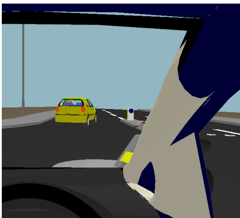
Figure 286. The scooter can effectively travel the whole distance until the point of impact obscured by the M 1 A-pillar – driver's view at point of impact
