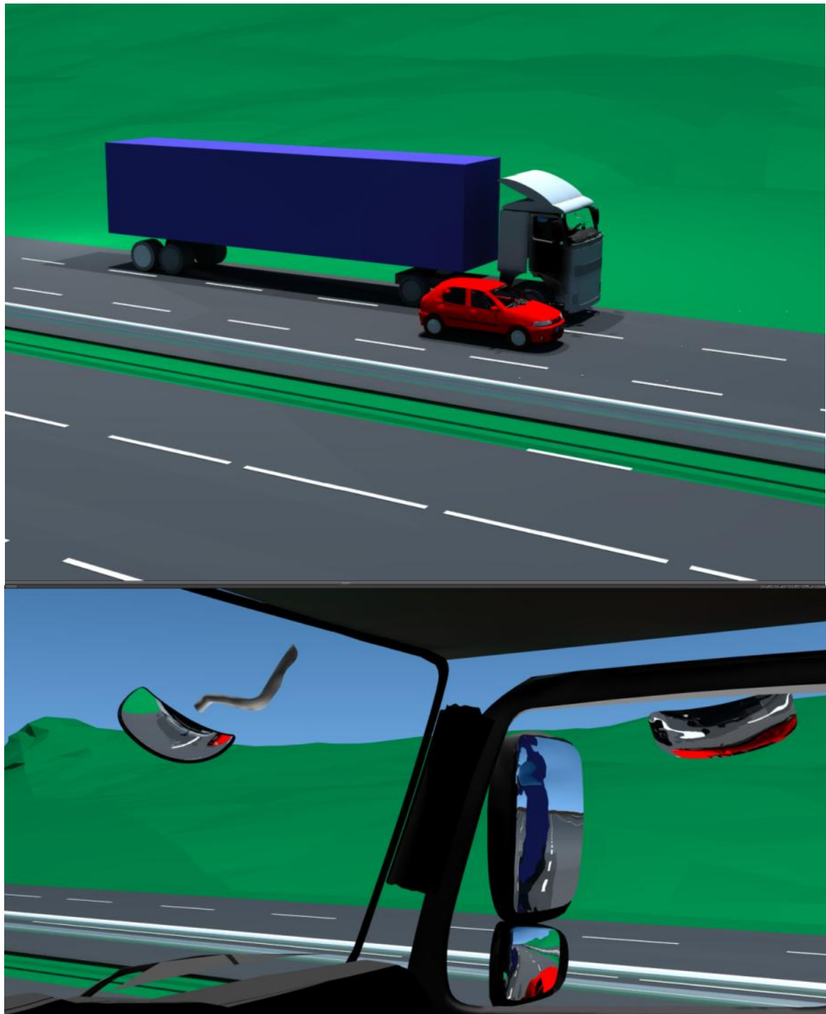
Figure 157. Stage 3: The vehicle is partially visible in the Class IV mirror and partially visible in the Class V mirror and Class VI mirror
