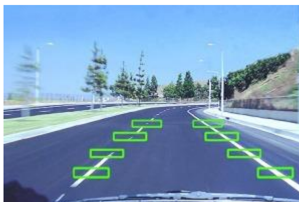
Figure 175. Tracking of Lane Markers by the Iteris Auto Vue LDWS
