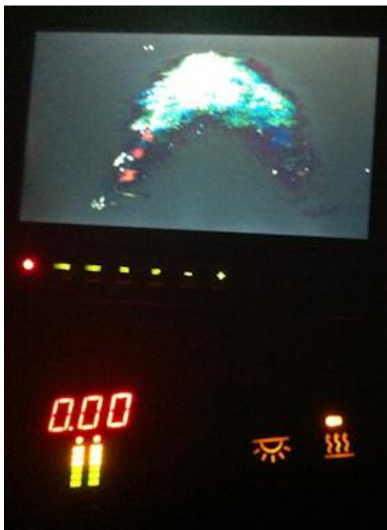
Figure 570. Class VI area sensor detecting target not visible on screen
