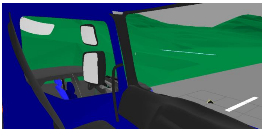
Figure 146. A car to the left of the driver's cab, and forward of the volume of space covered by the Class IV mirror is directly visible to a 99 th ile stature LGV driver
