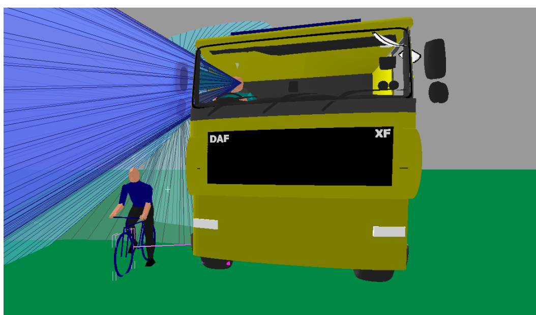
Figure 58. A 50 th ile UK female cyclist that is 950mm from the driver's side of the vehicle can be obscured from the 4 th ile stature driver
