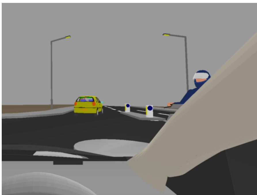
Figure 279. The scooter can effectively travel the whole distance until the point of impact obscured by the M 1 A-pillar – driver's view at point of impact
