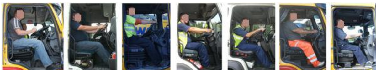
Figure 13. The variety of driver postures exhibited by drivers with a 4 th ile to 99 th ile stature range using UK anthropometric data (ADULTDATA 1998)
