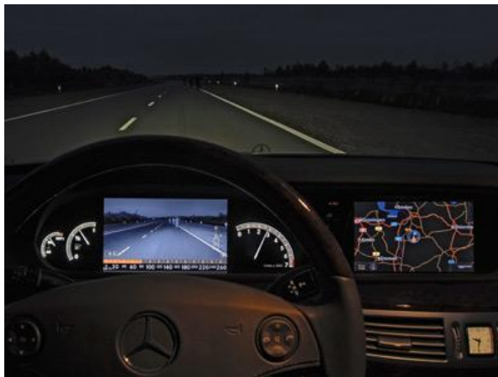
Figure 173. Mercedes Night View Assist Instrument Panel Display
