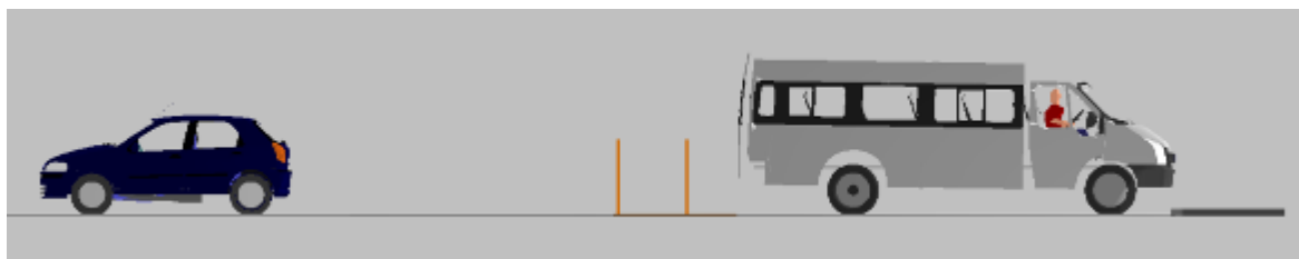
Figure 428. Rearwards visibility test A for 1100mm rearwards target (side view)
