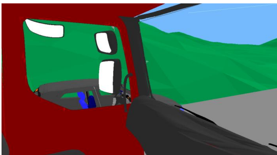
Figure 136. A car to the left of the driver's cab, and forward of the volume of space covered by the Class IV mirror is directly visible to a 4 th ile stature LGV driver
