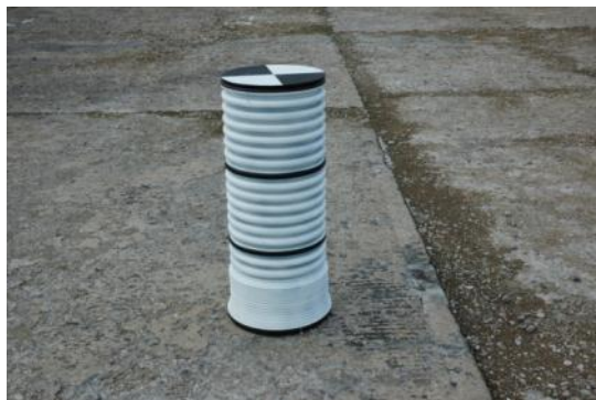
Figure 542. Test target used to validate prescribed field of view
