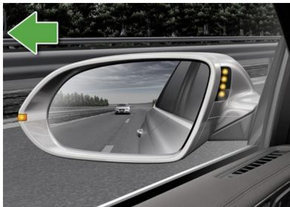
Figure 176. Lane Change Assistant Warning Next to Mirror
