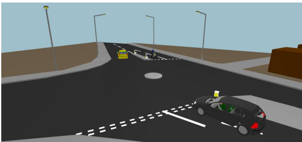
Figure 263. The roundabout layout showing the VW Golf and 99 th %ile Dutch male driver
