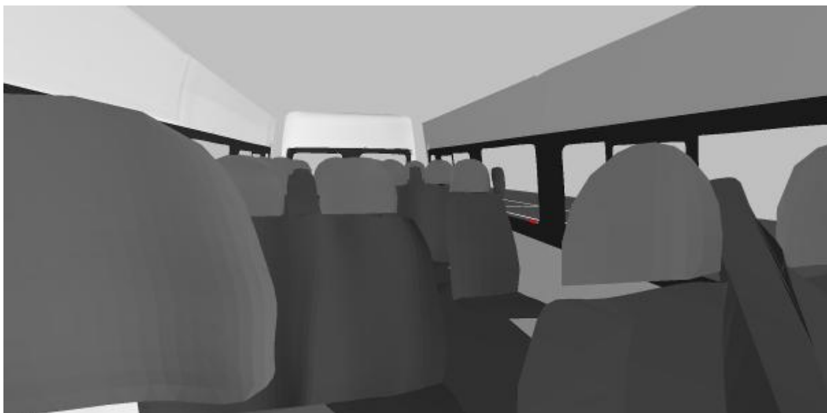
Figure 465. 1m Target Rearwards visibility unoccupied (head restraints at lowest setting)
