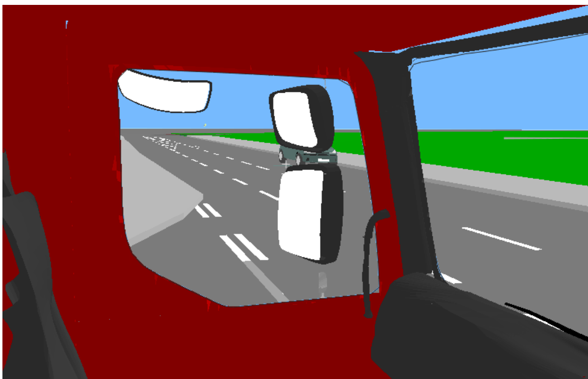
Figure 122. The driver's eye view: The approaching vehicle being partially obscured from the category N 2 Driver's vision due to the Class II and Class IV mirror surrounds
