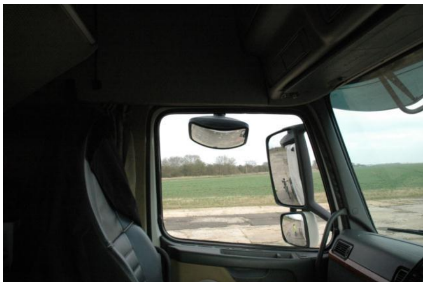
Figure 550. Spafax mirror mounted in Class V mirror position
