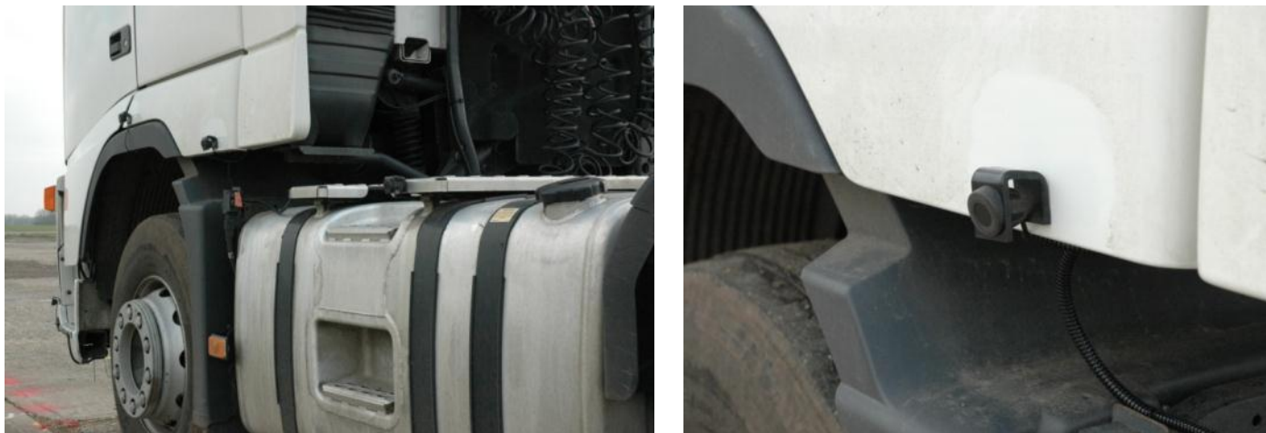
Figure 554. Sensors fitted to the side of the vehicle
