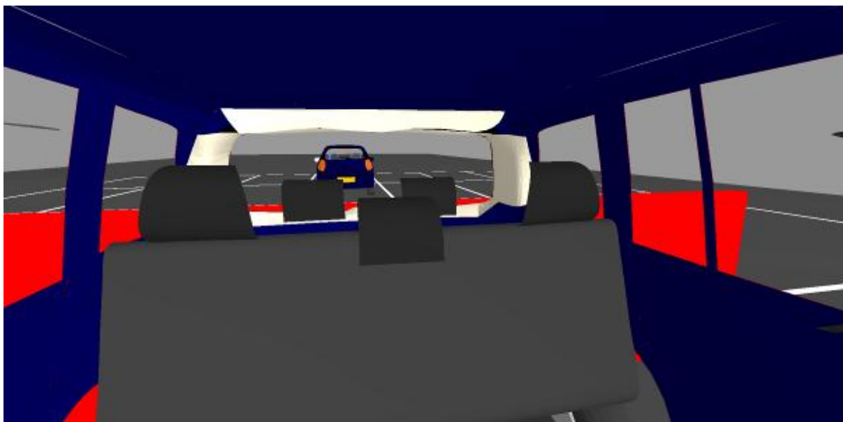
Figure 494. 1.15m Target Rearwards visibility unoccupied (head restraints at lowest setting)
