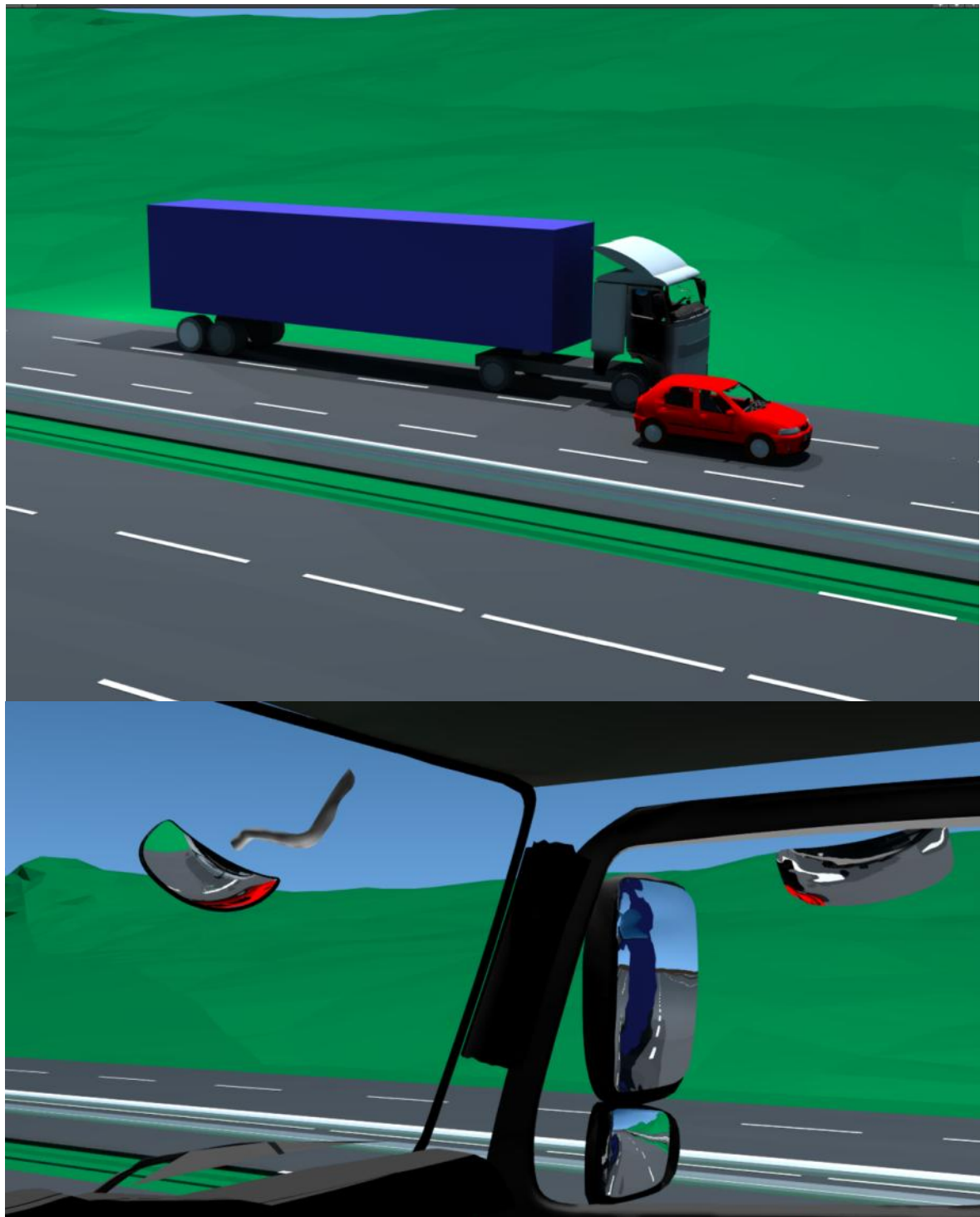
Figure 159. Stage 5: The vehicle is partially visible in the Class V mirror and Class VI mirror
