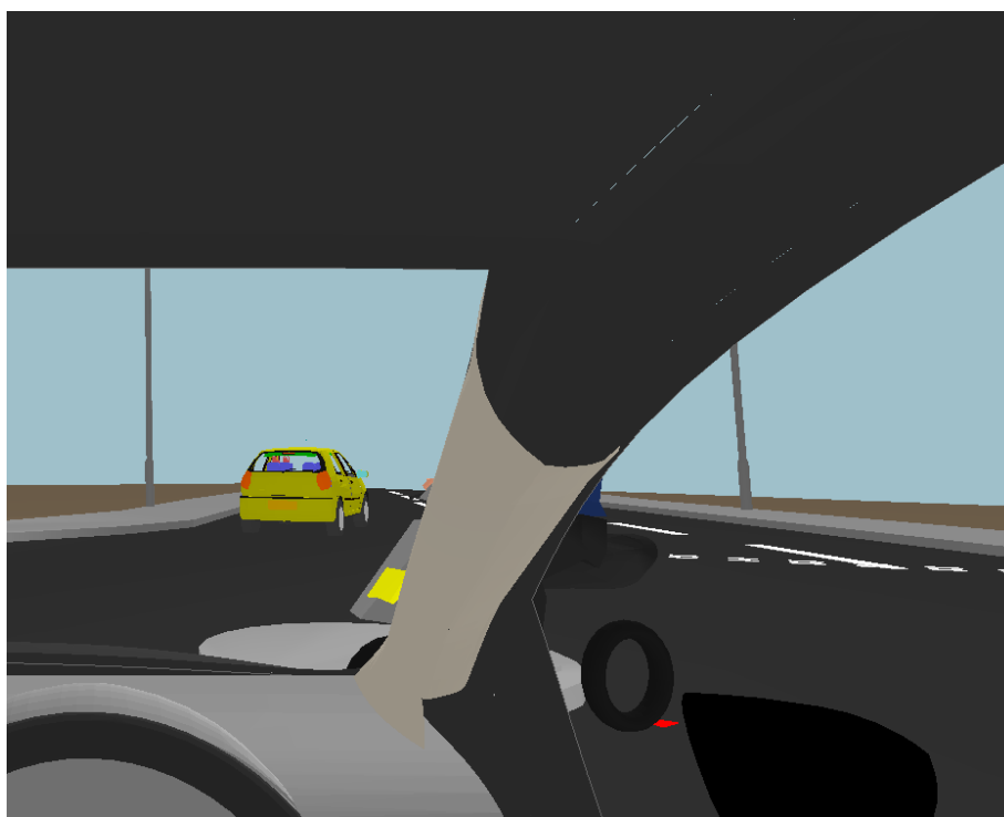
Figure 273. The scooter can effectively travel the whole distance until the point of impact obscured by the M 1 A-pillar – driver's view at point of impact
