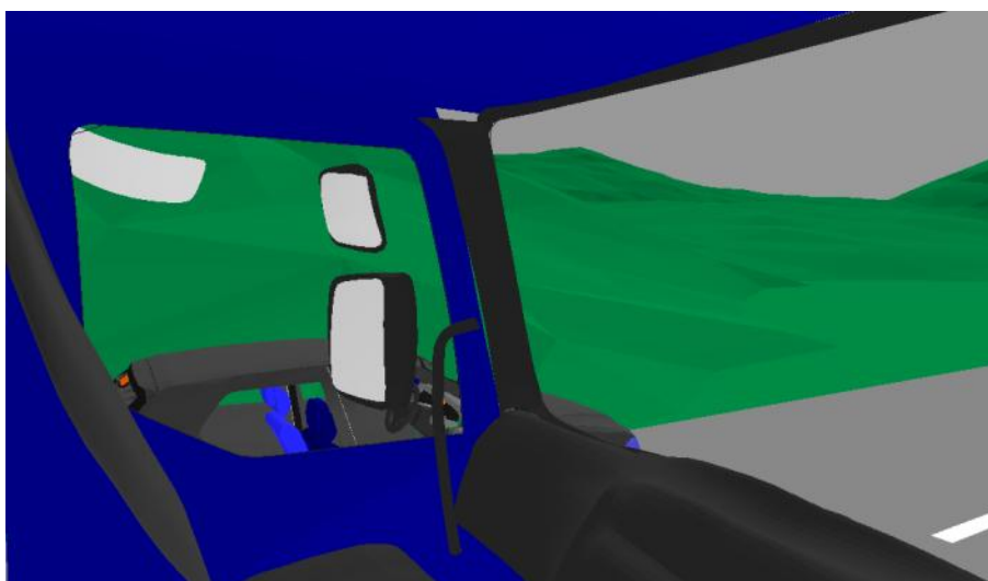
Figure 144. A car to the left of the driver's cab, and forward of the volume of space covered by the Class IV mirror is directly visible to a 4 th ile stature LGV driver
