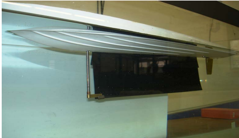
Figure 3. Under-water view of the hull and the assembled propulsive plate.
