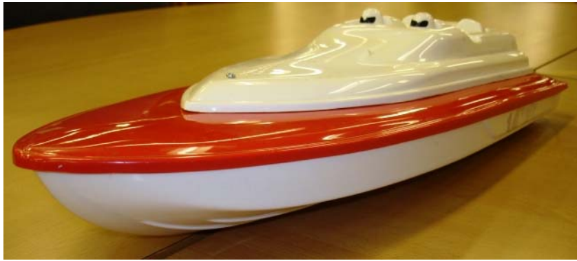
Figure 1. Hull assembly of the model boat
