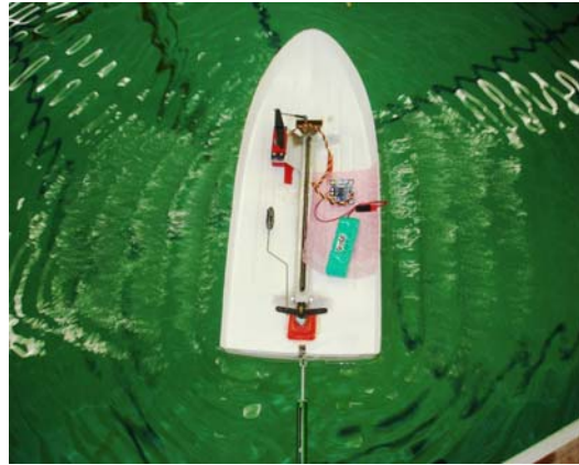
Figure 6. Static thrust test in progress
