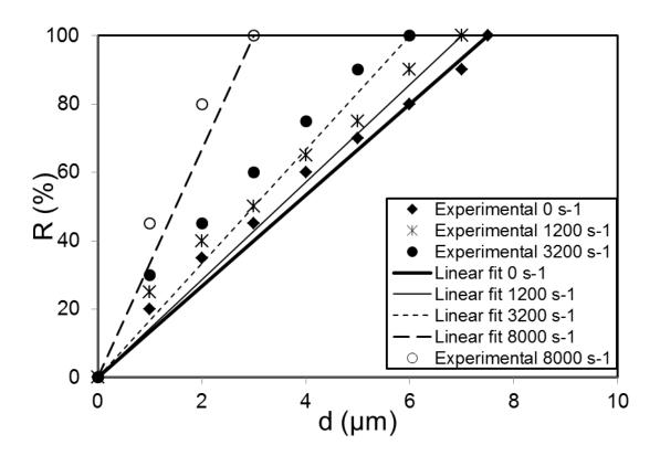
Fig. 9. (a) Rejection of crude oil droplets at flux rate (200 l m<sup>-2</sup> hr<sup>-1</sup>) and various shear rates (0, 1200, 3200, 8000 s<sup>-1</sup>).
