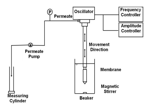
Fig. 4. Schematic view of vibrating microfiltration rig
