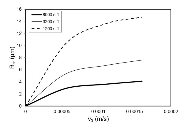
Fig. 6. Predicted drop size that would not reach the surface of the membrane due to migration velocities created by the fixed applied shear rate according to Eq (8).
