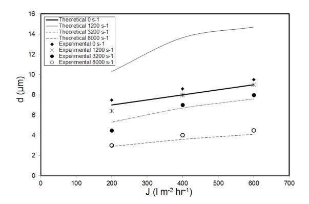
Fig. 8. Experimental measurements and theoretical points of 100% cut-off during filtering of crude oil droplets (22°A) at various shear rates (0, 1200, 3200, 8000 s<sup>-1</sup>) with different flux rates (200, 400 and 600 l m<sup>-2</sup> hr<sup>-1</sup>).
