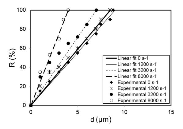
Fig. 9. (b) Rejection of crude oil droplets (22°A) at flux rate (400 l m<sup>-2</sup> hr<sup>-1</sup>) and various shear rates (0, 1200, 3200, 8000 s<sup>-1</sup>).
