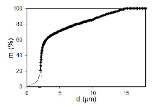
Fig. 5. Typical size distribution (Cumulative mass undersized "m" against droplet diameter "d") of the crude oil droplets (22°API).
