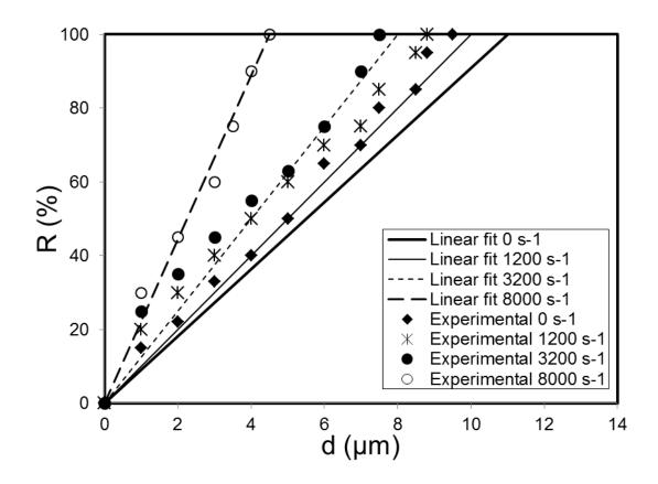
Fig. 9. (c) Rejection of crude oil droplets at flux rate (600 l m<sup>-2</sup> hr<sup>-1</sup>) and various shear rates (0, 1200, 3200, 8000 s<sup>-1</sup>).
