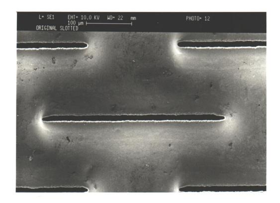
Fig. 3. Image of the surface of a slotted pore membrane.
