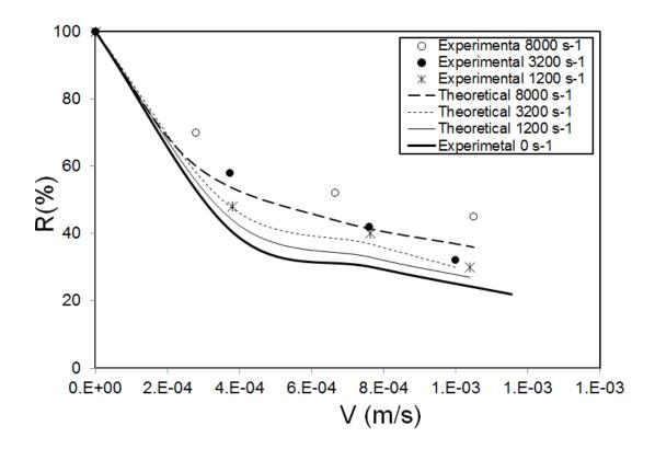
Fig. 7. Rejection (%) against filtration velocity (m/s) of 2 μm droplets at various shear rates according to the procedure presented in Fig. 2.
