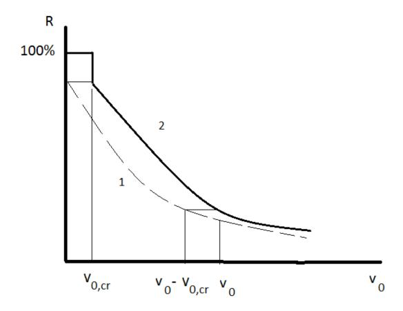
Fig. 2. 1- rejection curve when the shear rate is not applied. 2- calculations of the rejection according to the described procedure (see text).
