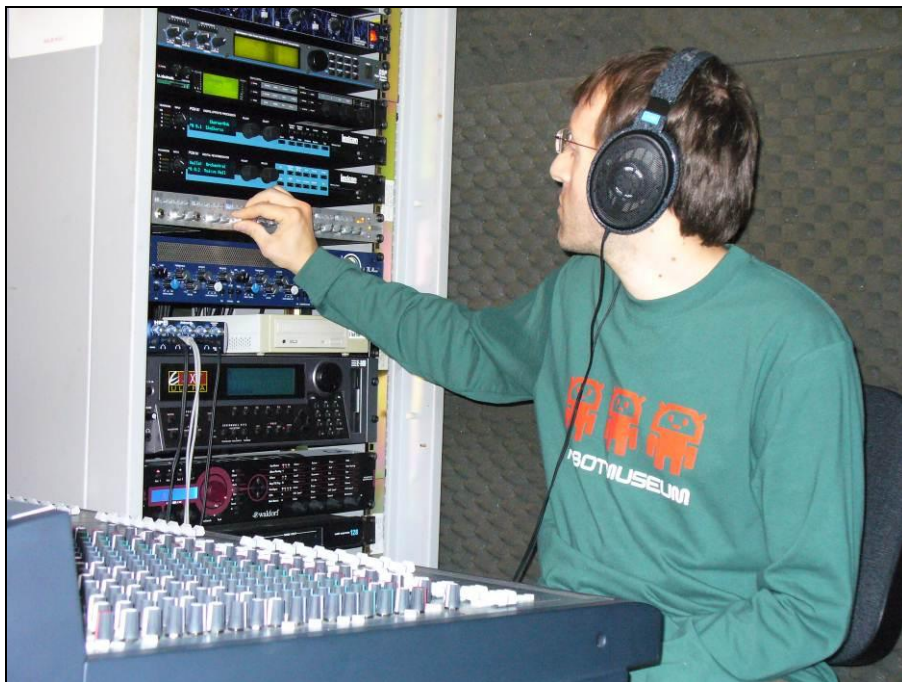
Figure 5-14: A studio engineer adjusting the input level on a microphone preamplifier during a recording session
