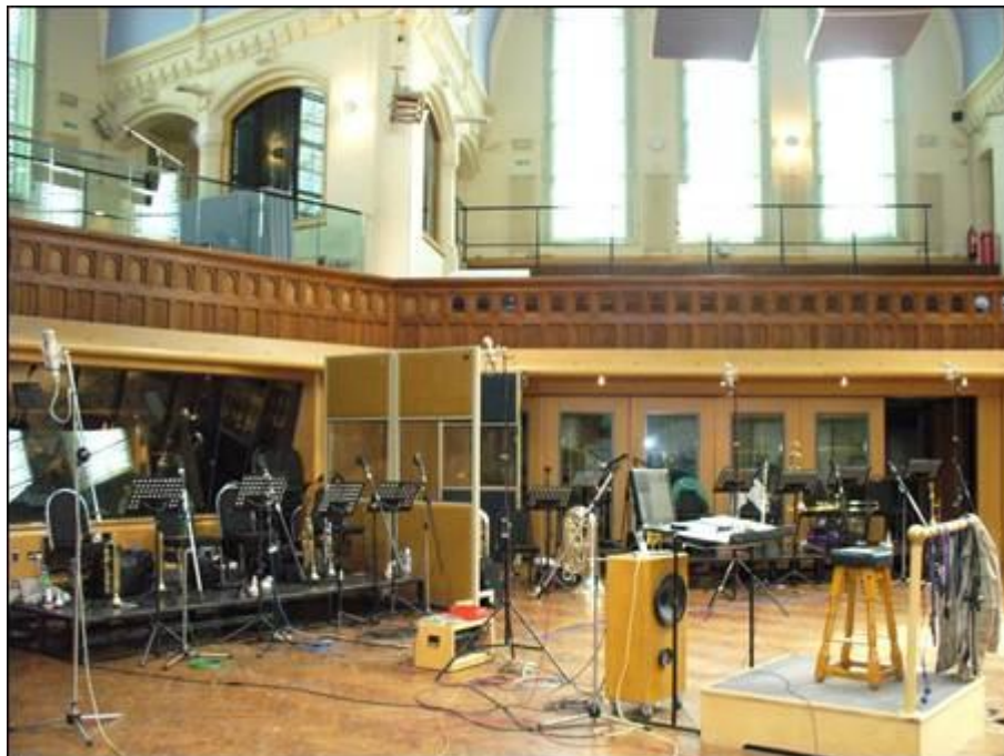
Figure 5-12: Microphoning for orchestral recording in a large acoustic space, Lyndhurst Hall, Air studios, North West London
