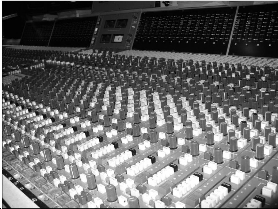
Figure 5-1: Close-up of recording console showing switches and faders for recording multiple tracks of audio, Fortress Studios, North London
