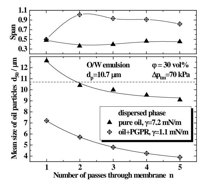
Fig. 6: The effect of the interfacial tension on the mean size and span of the particle size distribution in homogenized O/W emulsions (continuous phase: 0.5 wt% Tween 80 + 1 wt% Na-alginate + 5 wt% glucose; dispersed phase: pure soybean oil or 5 wt% PGPR in soybean oil). The mean pore size is designated by the dashed line.
