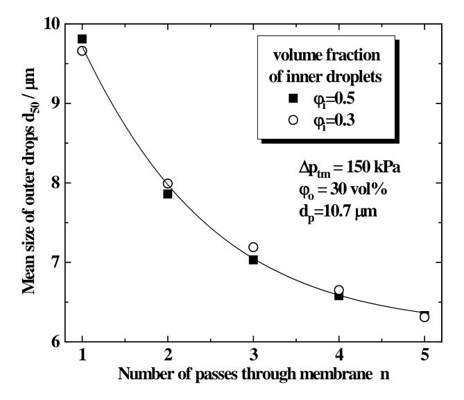
Fig. 3: The effect of volume fraction of inner droplets on the mean size of outer drops in product emulsions.
