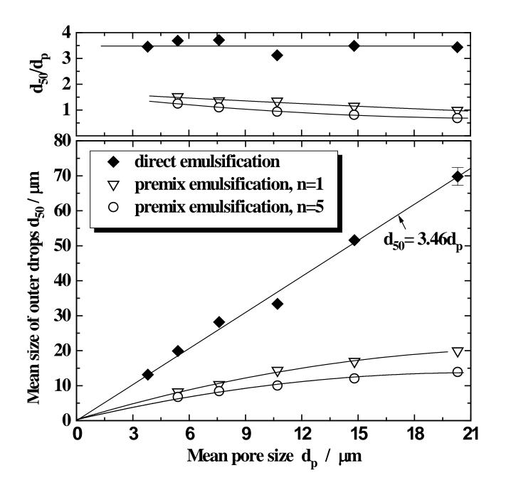
Fig. 11: The relationship between the mean droplet size and the mean pore size for multiple emulsions prepared using direct stirring membrane emulsification (stirring rate = 400 rpm) and repeated premix emulsification ( $\sigma_{w,pore} = 200$  Pa).
