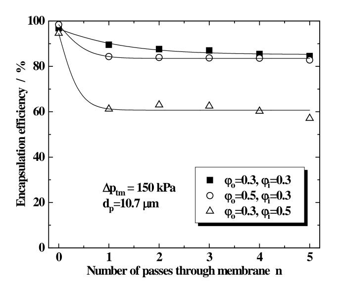
Fig. 2: The variation of encapsulation efficiency with the number of passes through the membrane at different volume fractions of inner ( $\phi_i$ ) and outer ( $\phi_o$ ) droplets.
