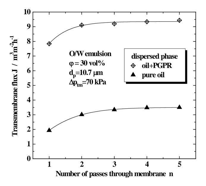
Fig. 7: The effect of the interfacial tension on the transmembrane flux (the experimental conditions as in Fig. 6).
