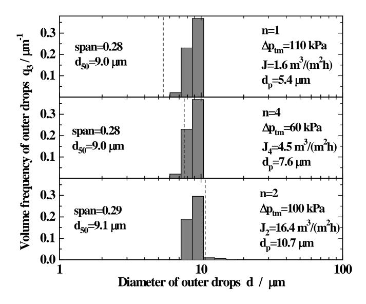
Fig. 12: The size distribution of outer drops prepared using SPG membranes with different mean pore sizes under such conditions to obtain almost the same
