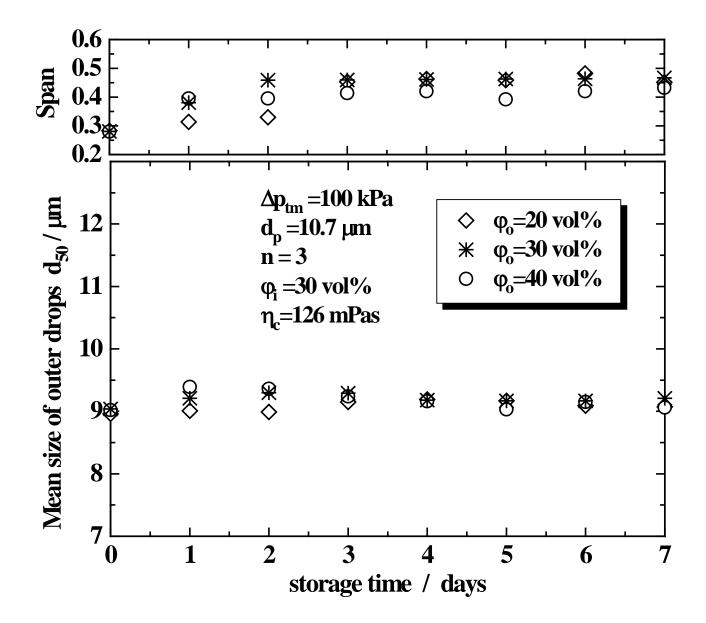
Fig. 14: The variation of the mean particle size and the span of particle size distribution of outer droplets during storage of multiple emulsions with different dispersed phase contents for one week at room temperature.
