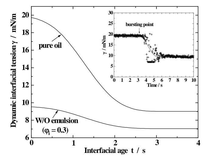
Fig. 5: Dynamic interfacial tension at oil-aqueous phase interface for two different compositions of oil phase (pure soybean oil or a W/O emulsion containing 5 wt% PGPR in soybean oil as a continuous phase). The aqueous phase in both cases was 0.5 wt% Tween 80 + 5 wt% glucose in bi-distilled water. The experimental  $\gamma$  vs. t data for pure oil are shown in the inserted figure.
