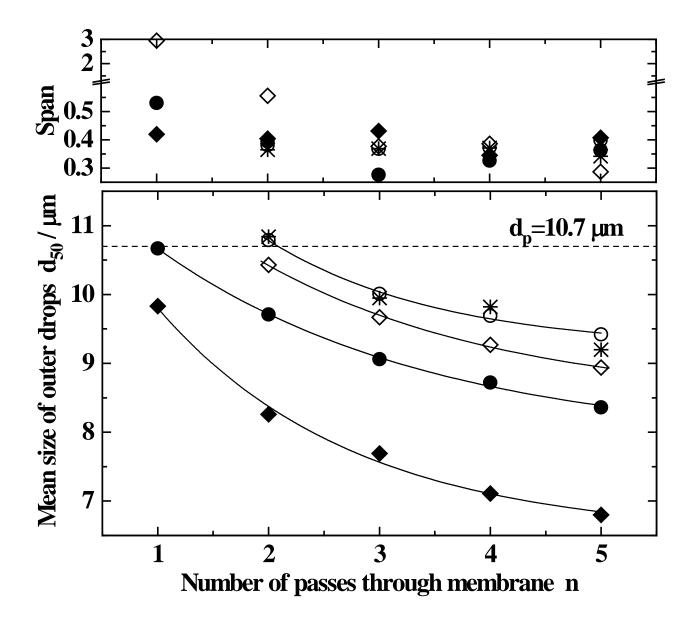
Fig. 9: The effect of the continuous phase viscosity on the mean size of outer drops. The symbols and experimental conditions are the same as in Fig. 8.
