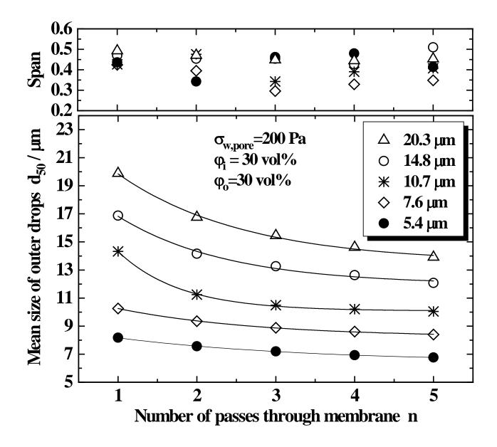
Fig. 10: The effect of the mean pore size on the mean droplet size at the constant shear stress of continuous phase inside pores of approximately 200 Pa ( $\eta_c = 126$  mPas).
