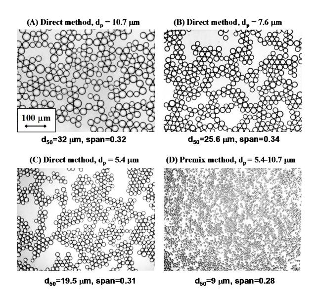
Fig. 13: The micrographs of droplets produced by direct and repeated premix emulsification using SPG membrane with a pore size of 5.4, 7.6, and 10.7  $\mu$ m. In the case of premix emulsification (D), the emulsions with the same particle size distribution can be produced, as shown in Fig. 12.
