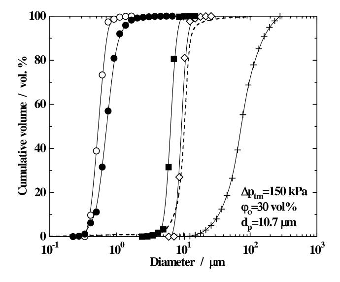
Fig. 4: Particle size distribution of emulsion droplets: (+) outer drops in feed emulsion; ( $\diamondsuit$ ) outer drops in product emulsion after a single pass; ( $\blacksquare$ ) outer drops in product emulsion after five passes; ( $\bullet$ ) inner droplets at  $\phi_i = 0.5$ ; ( $\bigcirc$ ) inner droplets at  $\phi_i = 0.3$ . Pore size distribution of the SPG membrane used is shown by a dashed line.
