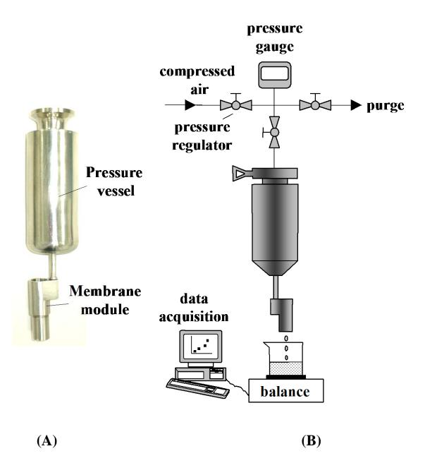
Fig. 1: (A) Membrane homogenizer used in this work. (B) Schematic view of experimental setup.
