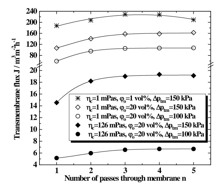
Fig. 8: The effect of the continuous phase viscosity on the transmembrane flux at two different pressures (100 and 150 kPa) and the contents of outer droplets (1 and 20 vol%). Other conditions:  $\phi_i = 30$  vol%,  $d_p = 10.7 \mu m$ .
