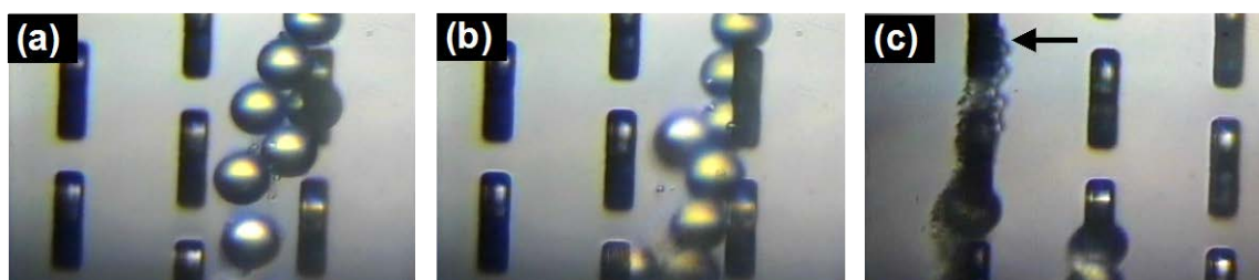
Fig. 6(a) and 6(b): Formation of satellite droplets at 1 wt% SDS; Fig. 6(c): Direct formation of small droplets from a channel clogged by dust particles. The location of this channel is marked by arrow.
