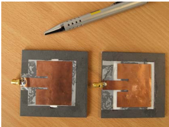
Figure 2. (a) 8mm wide slot at center of patch and (b) two 8mm wide slots at edges of patch.
