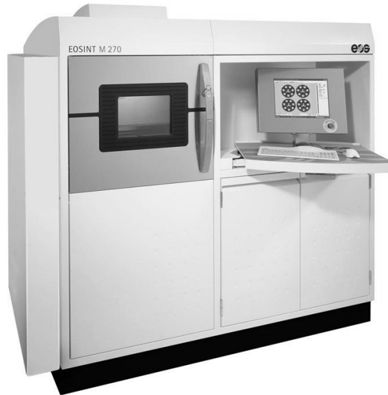
Figure 1: An example for an additive manufacturing system (EOSINT M270)
