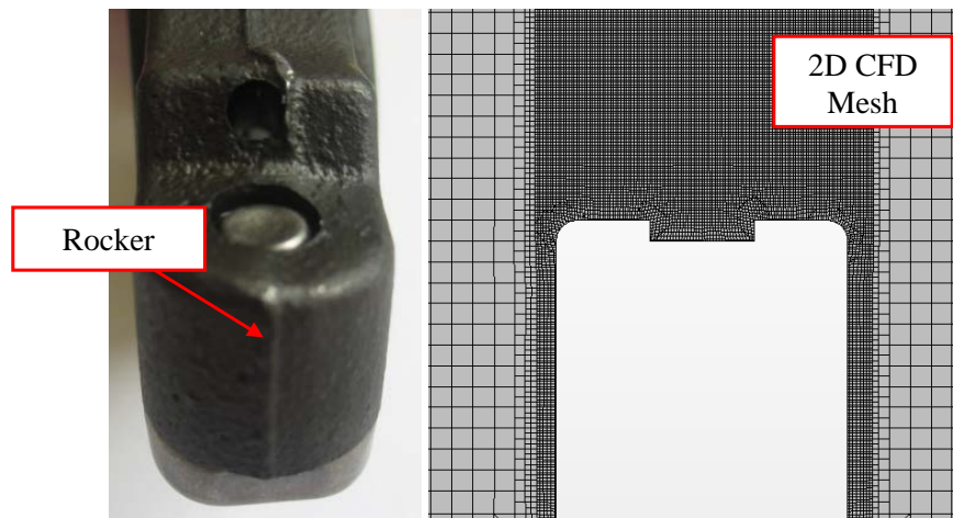
Figure 4.64 Rocker oil ligament breakup modelling (a) valve side of rocker (b) 2D CFD flow domain and mesh
