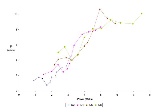
Fig. 6. Recorded speed v of the flow generated in a water tank by a localised wedge elastic wave propagating along the rubber plate as function of input electric power for different values of the wave displacement amplitudes; the amplitudes are identified by the locations of the holes on the motor disk: holes D2, D4, D6 and D8 correspond to the displacement amplitudes of 1.8, 2.2, 2.8 and 3.2 cm respectively.
