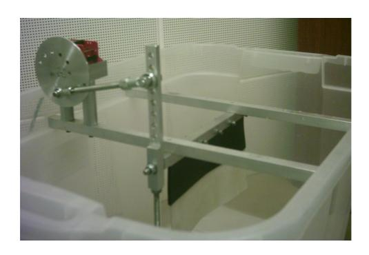
Fig. 3. View of the assembled propulsion rig in a an empty water tank used for in-tank testing: the main propulsive plate made of white rubber is stiffened by two narrower plates of black rubber; holes drilled on the motor disk are used for changing amplitudes of plate vibration.
