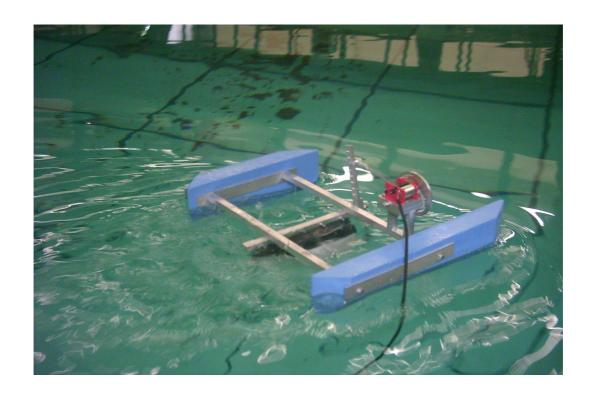
Fig. 8. View of the moving catamaran with wedge wave propulsive system during its testing in open water.
