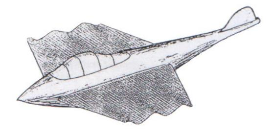
Fig. 1. On the proposed use of wedge elastic waves for propulsion of a small submarine [1]; the localised flexural waves propagate along the tips of the horizontal fins (wings), their energy being concentrated away from the main body.
