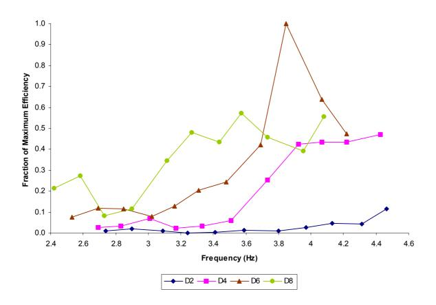
Fig. 7. Fraction of maximum efficiency of the process of flow generation in a water tank by a localised wedge elastic wave propagating along the rubber plate as function of frequency for different values of the wave displacement amplitudes; the amplitudes are identified by the locations of the holes on the motor disk: holes D2, D4, D6 and D8 correspond to the displacement amplitudes of 1.8, 2.2, 2.8 and 3.2 cm respectively.
