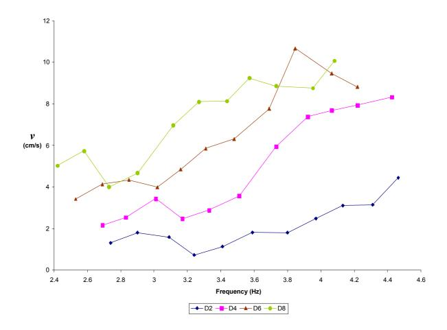
Fig. 5. Recorded speed v of the flow generated in a water tank by a localised wedge elastic wave propagating along the rubber plate as function of frequency for different values of the wave displacement amplitudes; the amplitudes are identified by the locations of the holes on the motor disk: holes D2, D4, D6 and D8 correspond to the displacement amplitudes of 1.8, 2.2, 2.8 and 3.2 cm respectively.
