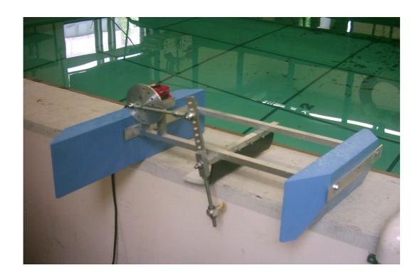
Fig. 4. View of the assembled catamaran with wedge wave propulsive system before its testing in open water.
