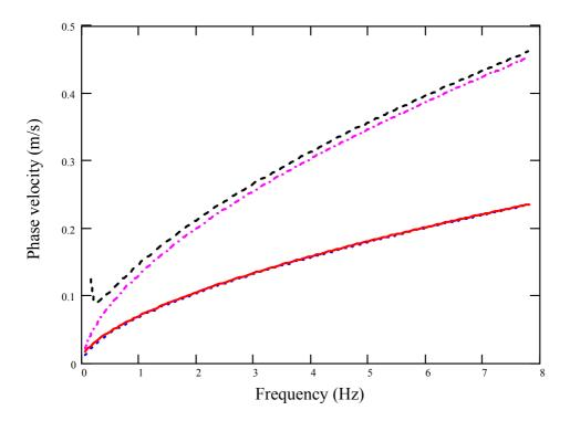
Fig. 2. Phase velocities of the lowest order flexural mode in two 'clamped-free' water-loaded rubber strips as functions of frequency; both strips are of the same width H = 150 mm, but have different values of thickness: h = 1 mm (solid curve) and h = 3 mm (dashed curve); for comparison, the velocities for infinite plates are shown for h = 1 mm (dotted curve, which practically coincides with the solid curve) and for h = 3 mm (dash-dotted curve).
