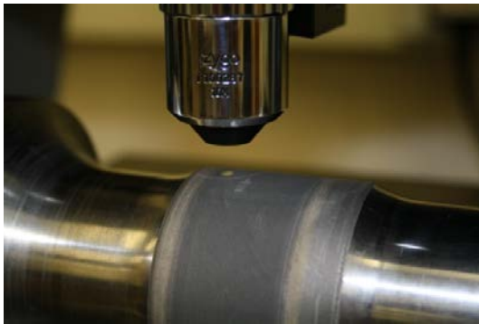
Figure 4-4: Photograph of the Zygo NewView™ 5000 white light interferometer used to measure the sonotrode weld surface texture.
