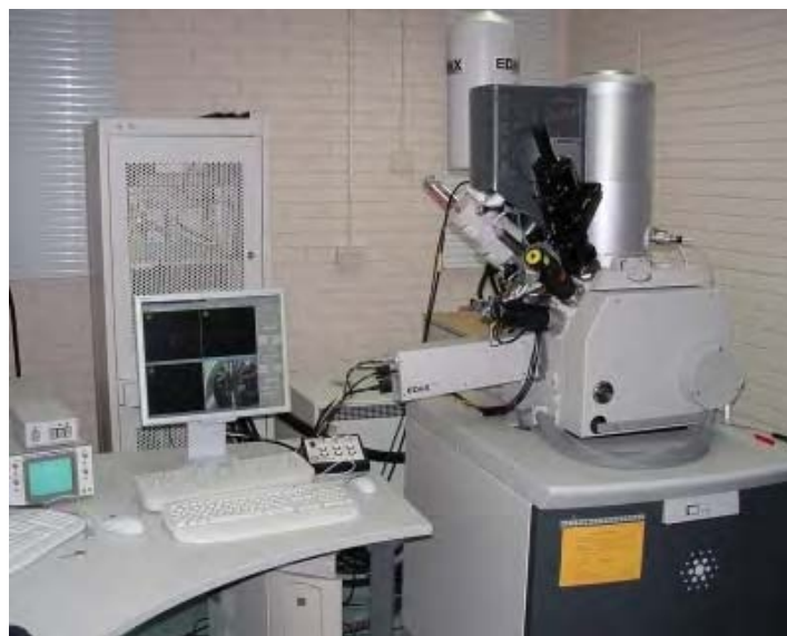
Figure 5-5: Nova 600 NanoLab, UHR FEG- DB SEM/FIB machine used to capture the FIB micrographs.
