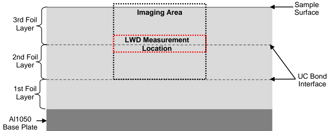
Figure 5-3: Diagram of UC sample cross-section illustrating a typical imaging area and the LWD measurement location.
