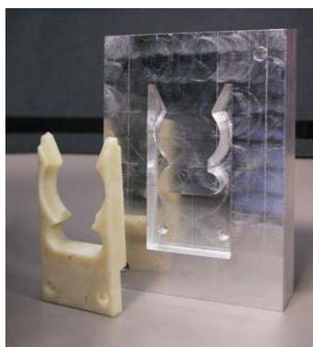
Figure 2-19: An example of a tool cast from a UC manufactured mould (White 2003).
