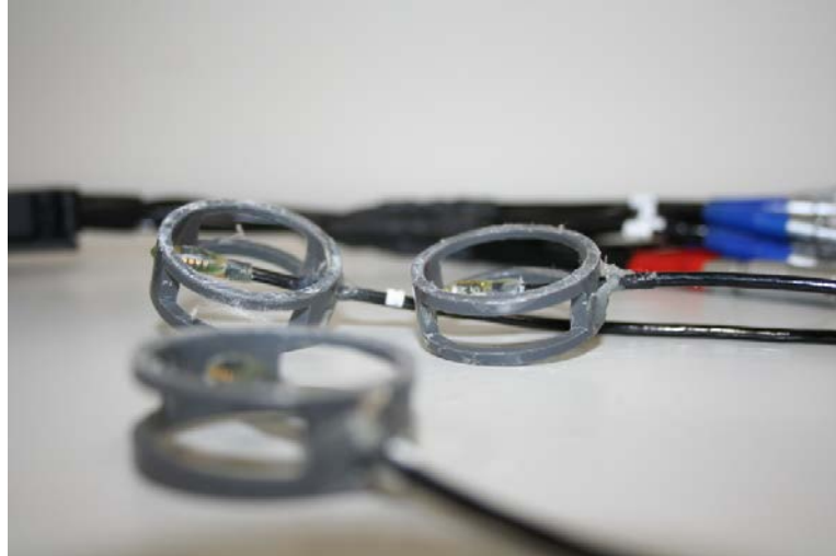
Figure 3.1: The MSR humidity sensors used to measure local skin wettedness. Each sensors is placed in a plastic holder to keep the sensor equal distance from the skin and clothing without restricting air movement around the sensor.
