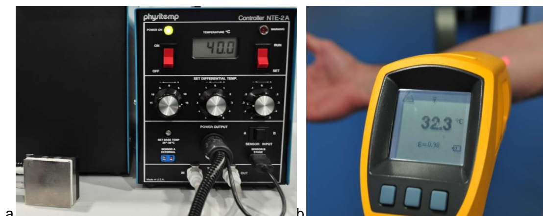
Figure 4.1: a) The thermal probe system set at 40°C. The metal square on the left hand side is the temperature controlled thermal probe. (b) The infrared thermometer used to measure pre stimulus skin temperature.
