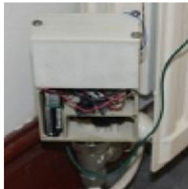
Figure 10.15 The thermal energy harvesting system with ZigBee Based Automatic Radiator
