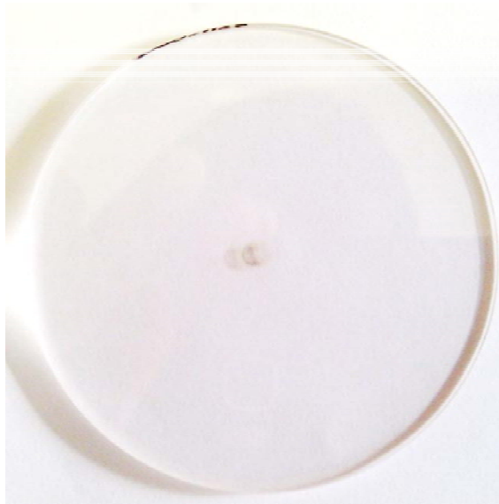
Figure 4.58: Deposition of soft, biological material on the non-contact cell window. In this figure, the material has been burnt into the window coating.
