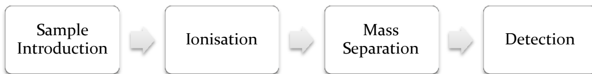
Figure 1.1: A simple schematic illustrating the stages involved in mass spectrometry. ‘Sample Introduction’ and ‘Ionisation’ may not necessarily occur in this order, e.g. using electrospray ionisation (see later), ionisation occurs before introduction into the mass spectrometer.
