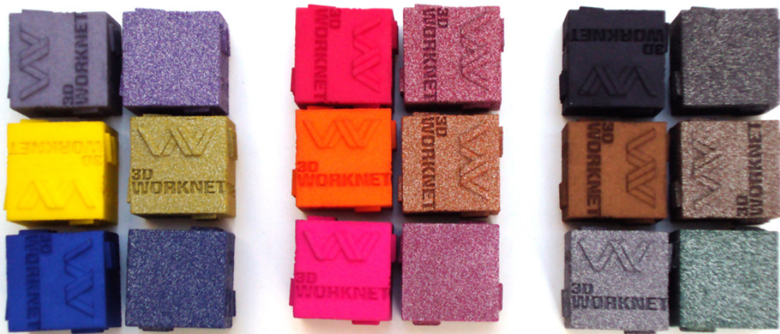
Figure 7. Dyed Alumine samples courtesy of 3D Worknet B.V.
