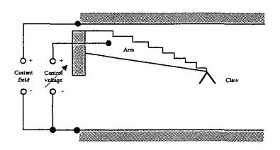
Fig. 17: Construction principle of a micro claw
