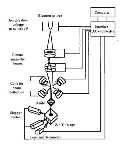
Fig. 3: Principle of an electron beam scanner/writer [Arno85]
