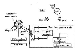
Figure 3: Data transmission system from AGV to host computer
