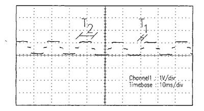
Fig. 36: Determination of the controller dead time
