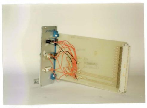
Photo 40: Side view of the photo detector II
