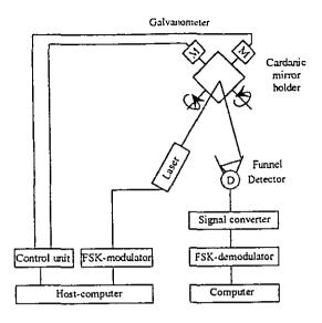
Figure 2: Data transmission system from host computer to AGV
