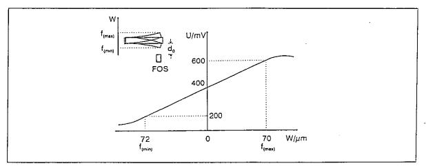
Figure 10: Dependence of the output signal from the FOS on the cantilever deflection, W, for a nominal displacement, d<sub>0</sub>, of 400µm
