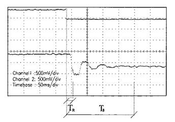
Fig. 31: Controlling characteristic of the focal position closed-loop control system
