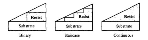
Fig. 1: Binary, staircase and continuous profile
