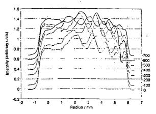
Fig. 10 Interference fringe structure from the FPE recorded with the photodiode array as a function of the distance from the centre of the ring pattern for each applied voltage
