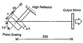
Fig. 6 Geometry of the dye laser resonator showing the effect of an expansion of the piezo ceramic parallel to the applied electric field
