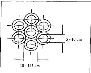
Figure 3: Principle of the fiber optical sensor (FOS) Figure 4: Cross-section of the FOS measuring
