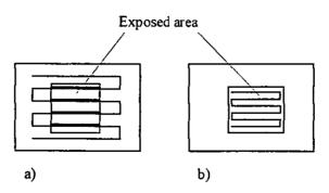
Fig. 50: Raster - and vector scanning methods
