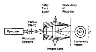
Fig. 8 Experimental set-up for the recording of FPE ring patterns
