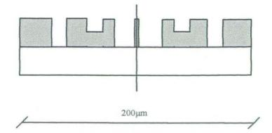
Fig. 58: Cross section of the expected multi level microstructure
