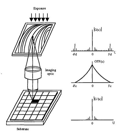
Fig. 10: Process principle of the binary raster scan method [Pole91]
