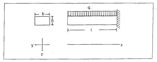
Figure 1: Cantilever model
