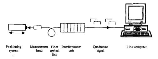
Fig. 33: Block diagram of the interferometer system [Grüb92]
