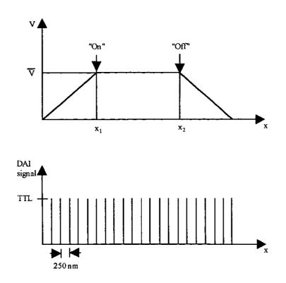
Fig. 34: Principle of the Direct Axis Interface
