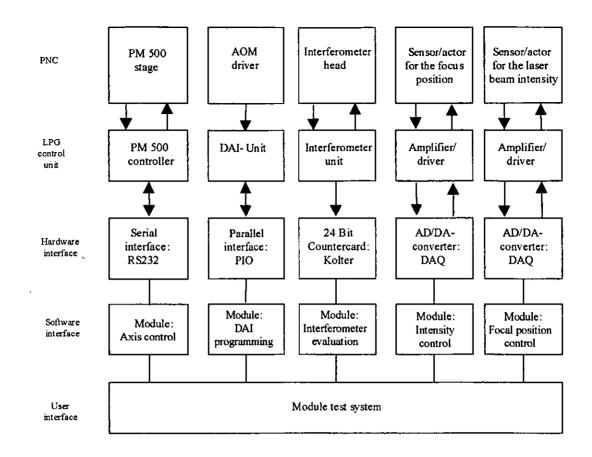
Fig. 37: Modules used in the test system
