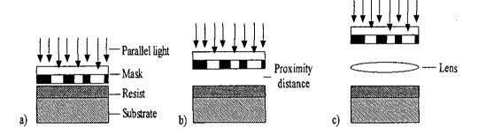
Fig. 6: Principles of mask transfer
