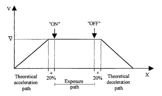
Fig. 45: vt-diagram of the CP - procedure
