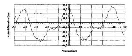
Fig. 41: Error curve of the positioning system
