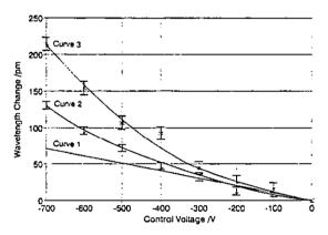
Fig. 11 Wavelength shift of the dye laser as a function of the voltage applied to the piezo grating. Curve 1: linear theory according to equation (6); Curve 2: calculated wavelength shifts, as expected from the experimentally determined grating constant data displayed in Fig. 4; Curve 3: average of the data obtained from the FPE measurements using photographic film and the diode array. (Curve: see note to Fig. 4)
