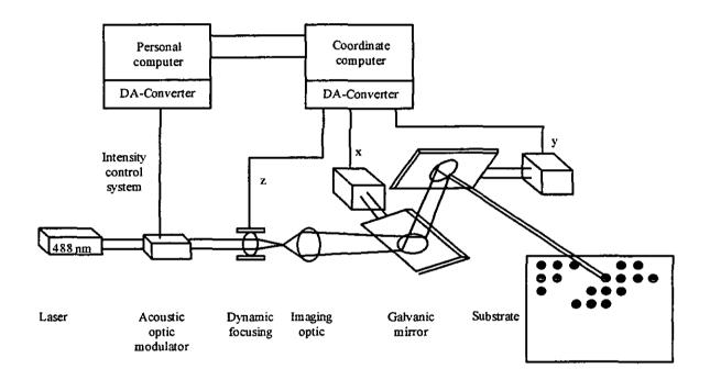
Fig. 4: Principle of a laser beam scanner [Jäge92]
