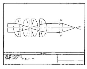
Figure 5: Raytracing model of the autofocus sensor
