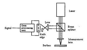
Figure 2: Modified autofocus sensor
