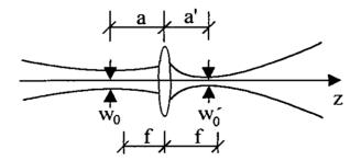
Fig. 22: Gaussian beam transformation by a lens
