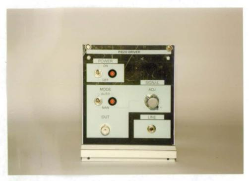
Photo D24: Front view of the piezo driver
