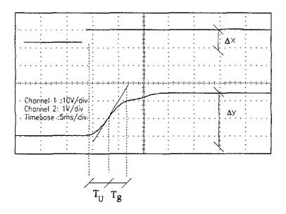
Fig. 30: Step response for the determination of the system parameter
