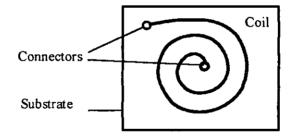
Fig. 19: Construction principle of a micro coil [Menz93]
