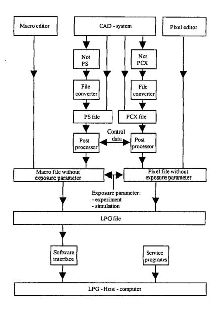
Fig. 48: Software concept for exposure programs
