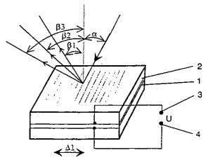
Fig. 1 Schematic representation of the reflection grating depicting various diffraction angles as a result of voltage tuning of the grating line spacing. The variation in  $\beta$  has been grossly exaggerated for clarity
