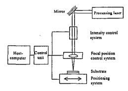
Figure 1: Principle set-up of the Laser Pattern Generator
