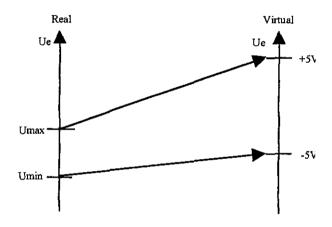
Fig. 35: Conversion of the input signal
