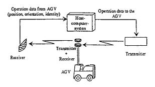
Figure 1: Schematic of a combined communication and navigation system
