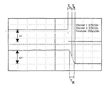
Fig. 25: Step response for the determination of the system parameter
