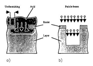
Fig. 12: Wet a) and dry b) etching process
