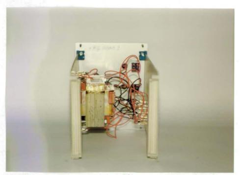
Photo D25: Back view of the piezo driver
