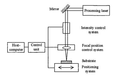
Fig. 20: Principle set-up of the Laser Pattern Generator
