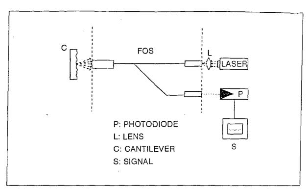
Figure 3: Principle of the fiber optical sensor (FOS)
