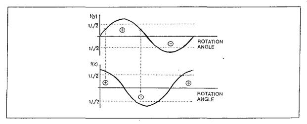
Figure 6: Bending of the cantilever as a function of the rotation angle
