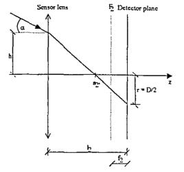
Figure A2: Geometry of the beam propagation between the lenses
