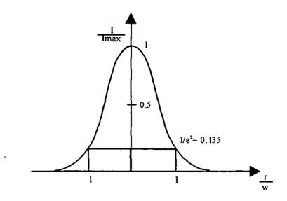
Fig. 52: Cross-section of a Gaussian beam
