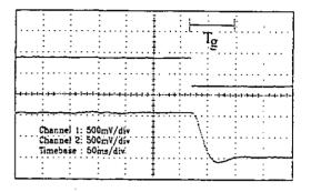
Figure 8: Response of the closed-loop system to a step of the set point
