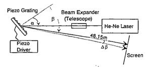
Fig. 3 Experimental set-up for the investigation of the tuning characteristics of the grating
