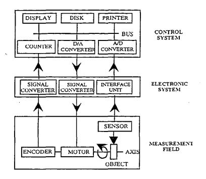
Figure 3: Block diagram of the automated roundness measurement system
