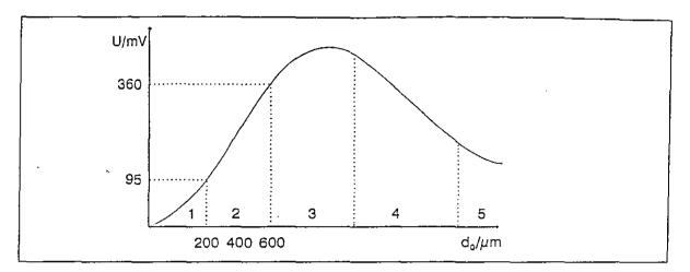
Figure 8: Output, S, of the FOS versus nominal displacement, d<sub>0</sub>, from the reflecting and scattering cantilever surface
