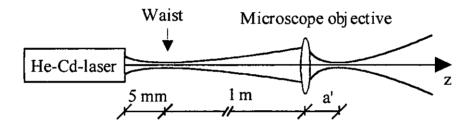
Fig. 21: Beam path of the exposure laser
