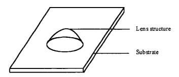
Fig. 13: Refractive microlens
