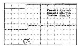
Figure 5: Response of the closed-loop system to a step of the set point
