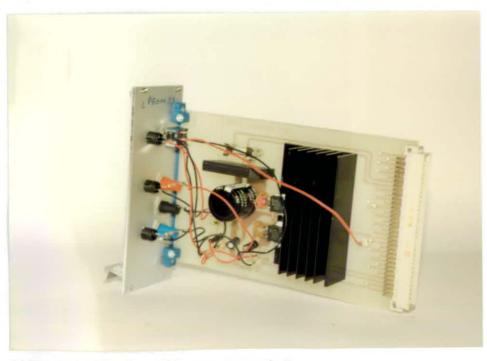
Photo D9: Side view of the power supply I
