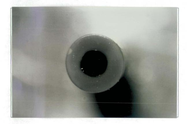
Fig. 64: Micro lens on the end of a fiber
