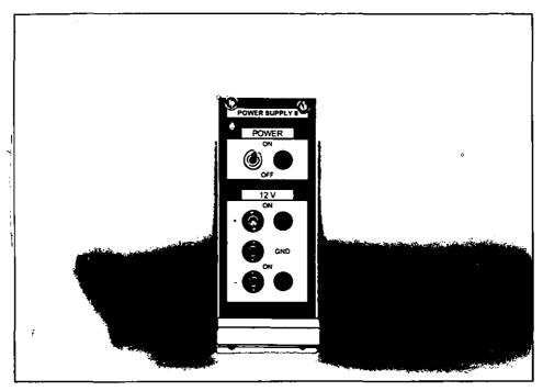
**Photo D10:** Front view of the power supply II
