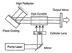
Fig. 5 Principle design of the dye laser with the piezo grating installed in a Littmann/Metcalf configuration
