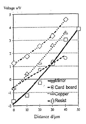
Figure 2: Measurement characteristics of the distance sensor
