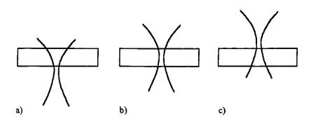
Fig. 53: Focal positions relatively located to the resist layer
