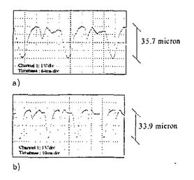
Figure 10: True running measurement
