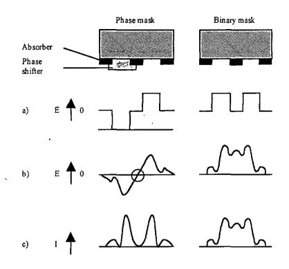
Fig. 9: Comparison between a phase mask and a binary mask
