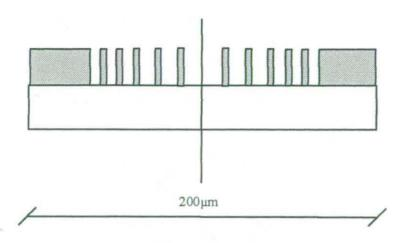
Fig:56: Cross section of the expected binary microstructure
