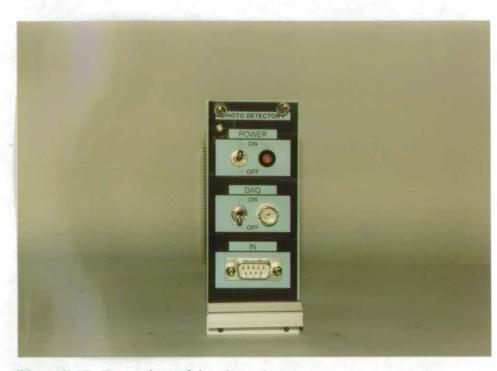
Photo D37: Front view of the photo detector I
