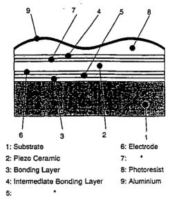
Fig. 2 Cross-section of the piezo grating
