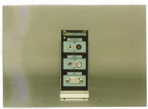
Photo D39: Front view of the photo detector II
