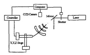
Figure 1: A complete laser cutting system for automatic plant propagation
