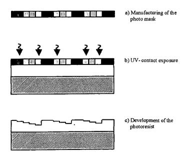
Fig. 11: Process principle of the grey level mask method [Ande90]
