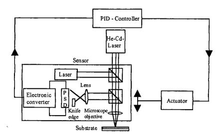
Fig. 28: Focal position closed-loop control system
