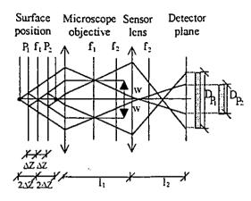
Figure 4: Beam path of the sensor
