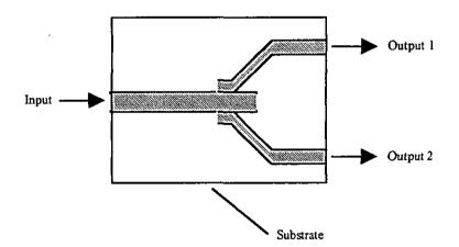
Fig. 15: Structure of a planar optical waveguide
