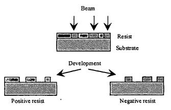
Fig. 51: Positive and negative resist
