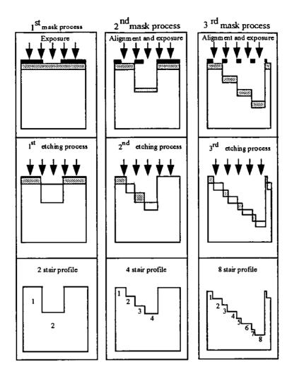
Fig. 8: Sequence of operation in a multiple mask process
