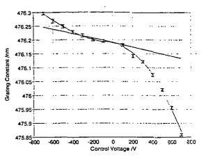
Fig. 4 Theoretically and experimentally determined grating constants as a function of the applied voltage. The curve drawn through the experimental data is to guide the reader's eye only and is not intended to represent any particular functional dependence
