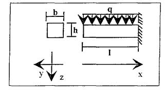
Figure 1: Cantilever model
