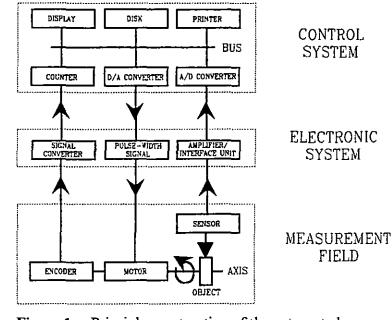
Figure 1: Principle construction of the automated system for roundness measurement
