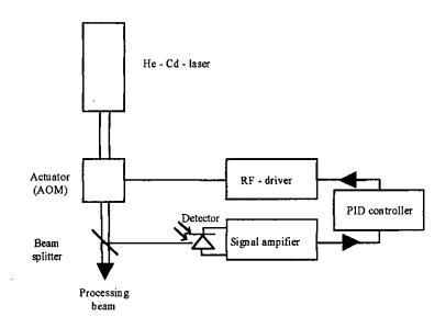
Fig. 23: Intensity closed-loop control system
