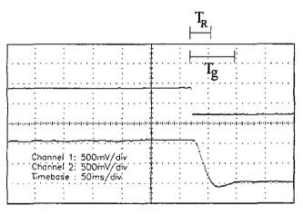
Fig. 26: Controlling characteristic of the intensity closed-loop control system
