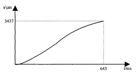
Fig. 39: st-diagram of the PM500
