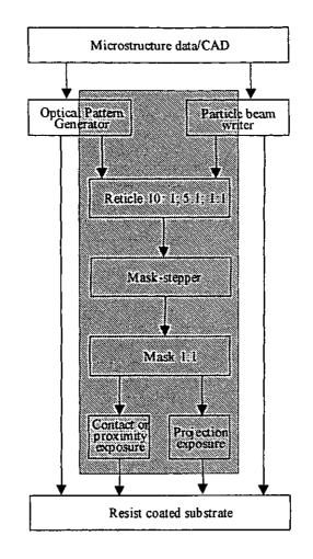
Fig. 2: Block diagram of microstructuring processes
