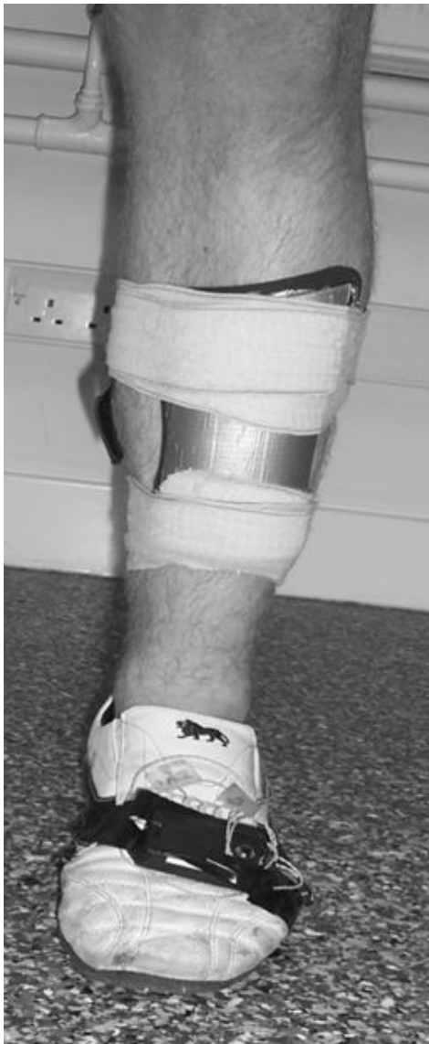
Figure 2. Positioning of the 0.9kg mass for the WC tests
