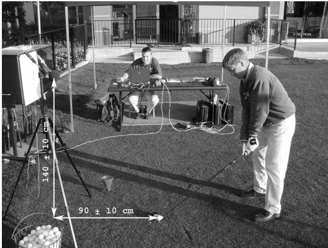
Figure 1. Microphone location in the test set-up
