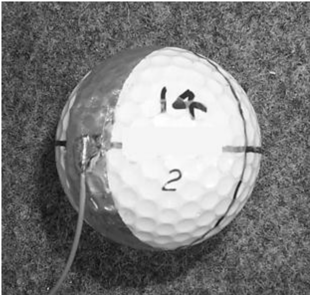
Figure 2. Wire soldered to a small patch of tape, with a conductive adhesive backing, attached to the surface of the conductive covering.
