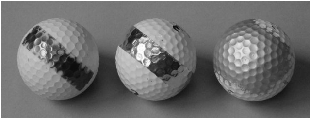
Figure 1. Three different techniques for applying conductive coating to a golf ball: from left to right, embedded copper strip, aluminium foil and silver conductive paint.
