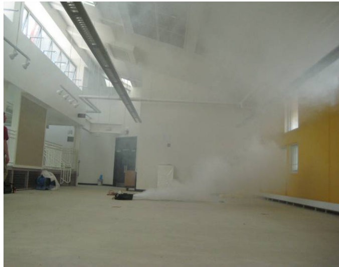
Fig 10: The level four studio showing the raised air inlet (left), the louvered control air outlet to the south-west most turret, the clerestory windows, the perimeter windows and the theatrical smoke machine
