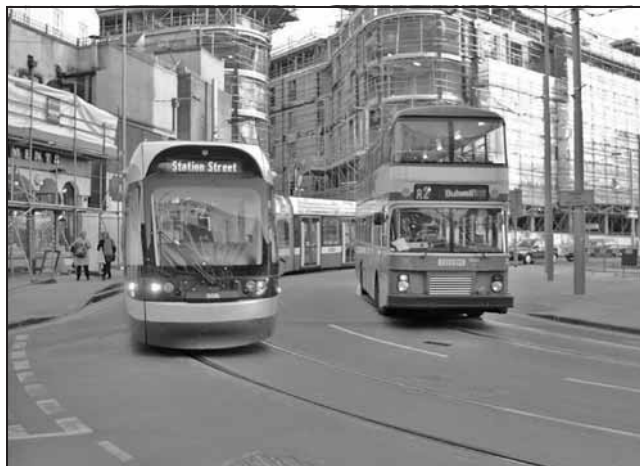
Fig. 3. Lace Market Curve and tram stop with a southbound tram and a bus waiting to turn right. Note: Lace Market Curve is the tightest curve on a UK tramway; the tram stop can be seen to the right of the picture. Buses pass through the stop and turn right on the curve to the junction in the foreground to the left of the picture
