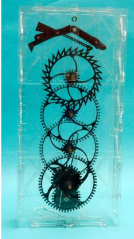
Figure 2 Grasshopper escapement and skeletonised gears
