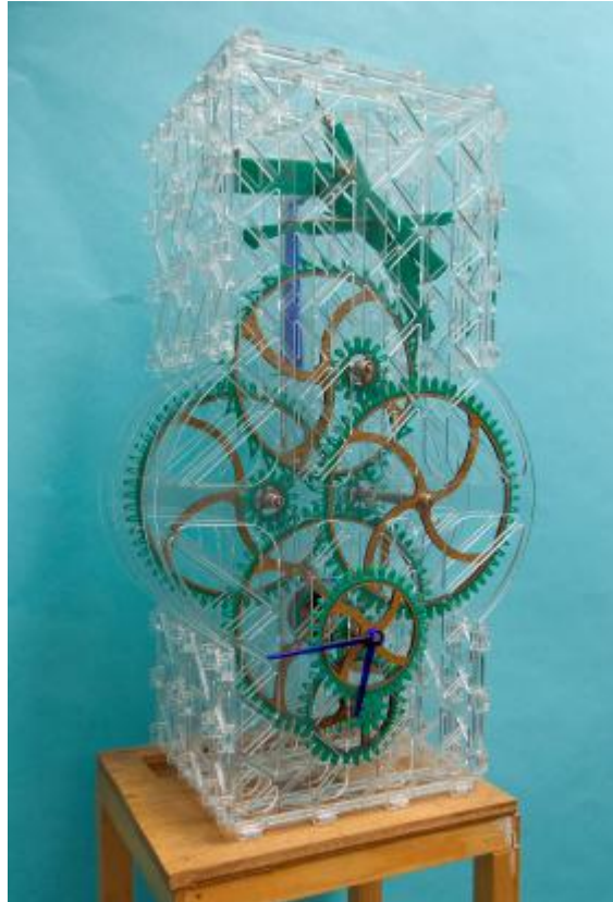
Figure 3 Grasshopper escapement with Acrylic and Kevlar gears
