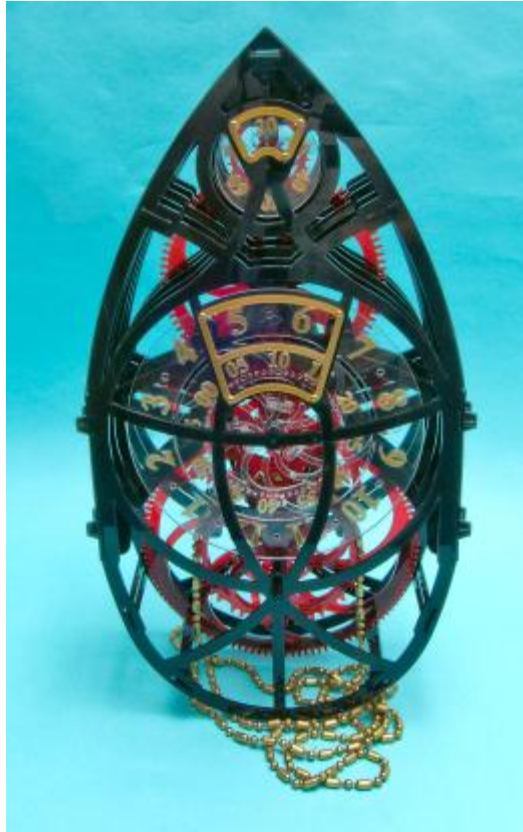
Figure 6 Geneva mechanisms create a digital face
