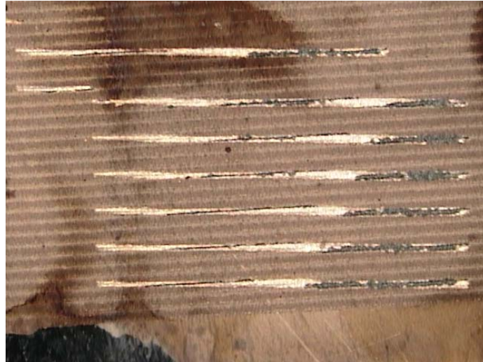
Figure 11. Premature plating failure as a function of stylus/discontinuity impact
