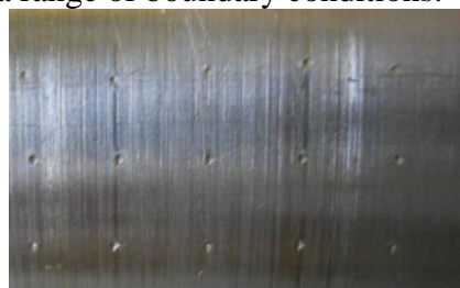
Figure 3: Distribution of surface dimples on the journal face
