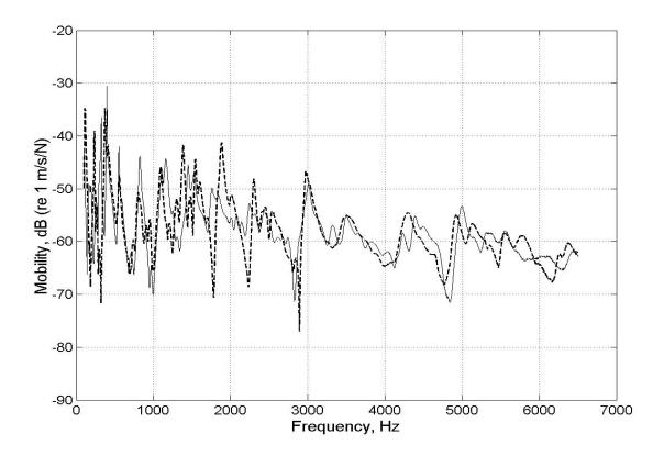
Fig. 6. Measured point mobility of a quadratic steel wedge covered by a thin strip of thickness  $\delta = 0.2$  mm (dashed curve) and by a thick (3-mm) adhesive layer (solid curve); the position of the shaker was at 100 mm from the thick end of the wedge and at 100 mm from both side edges.
