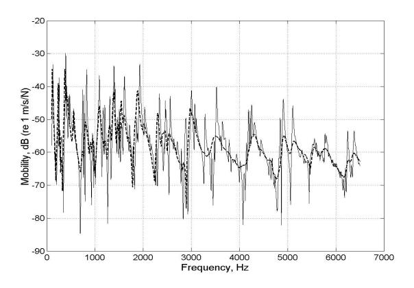
Fig. 4. Measured point mobility of a quadratic steel wedge: free wedge (solid curve) and wedge covered by a thin adhesive strip of the thickness  $\delta = 0.2$  mm (dashed curve); the position of the shaker was at 100 mm from the thick end of the wedge and at 100 mm from both side edges; note a significant suppression of resonant peaks in a wedge covered by an adhesive strip.
