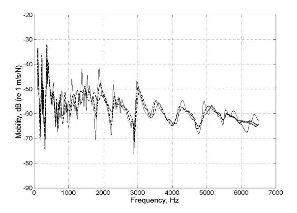
Fig. 5. Measured point mobility of a quadratic steel wedge covered by several thin adhesive strips of thickness  $\delta = 0.2$  mm each: one strip (solid curve), two strips (dashed curve) and three strips (dash-dotted curve); the position of the shaker was at 100 mm from the thick end of the wedge and at 100 mm from both side edges.
