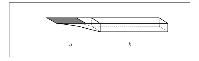
Fig. 1. Damping of resonant vibrations can be achieved by reducing wave reflections from edges of structures, in addition to a more traditional way of increasing local wave attenuation; in particular, one can apply a non-symmetric quadratic wedge-like damper covered by an absorbing film on one side (a) for suppression of flexural wave reflections from one of the edges of an elastic plate (b) [1-4].
