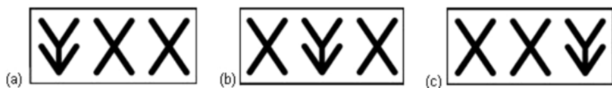
Figure 15.4 LCT signs: (a) left, (b) centre, (c) right (source: ISO 26022:2010, with permission)
