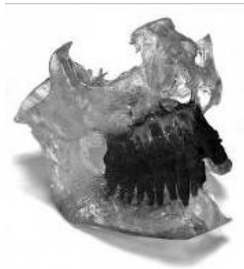
Figure 2: A typical medical model made by stereolithography.
