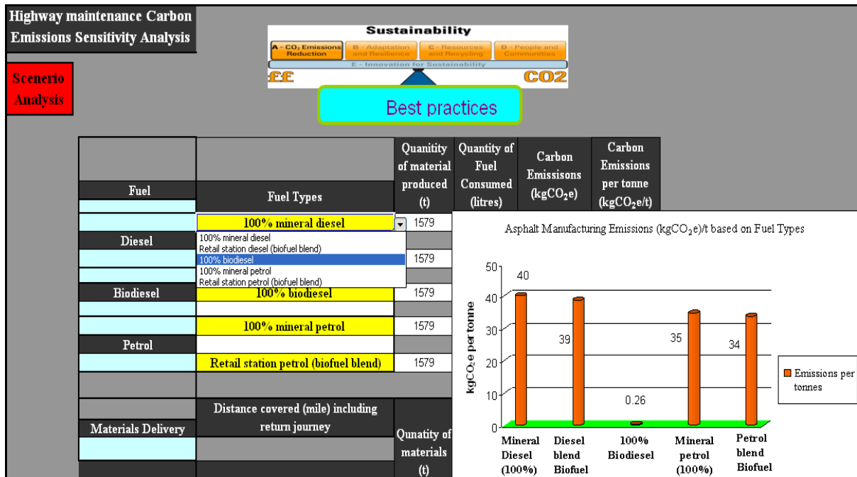
Figure 3. Asphalt manufacturing Emissions using different fuel types
