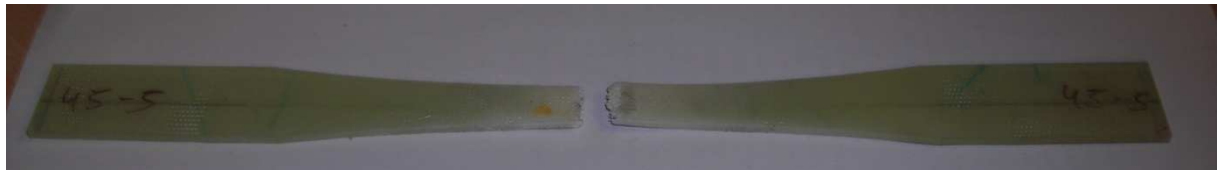
Figure 57: Fractured Dogbone Specimen
