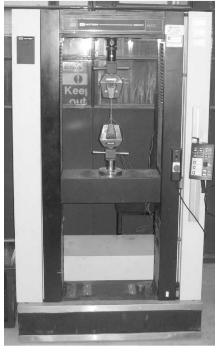
Figure 60: INSTRON 5500R-6025 universal testing machine
