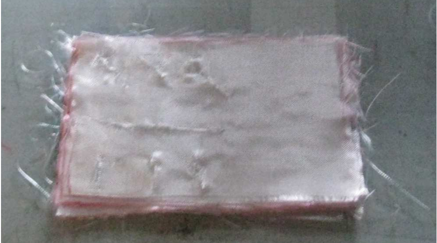
Figure 18: Dry Preform on Mould
