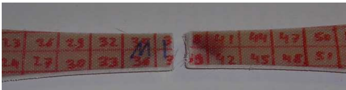
Figure 61: Fracture of Tensile Test Specimen
