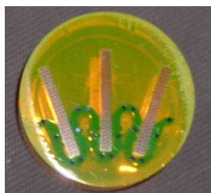
Figure 25: Polished Digital Microscopy Specimen
