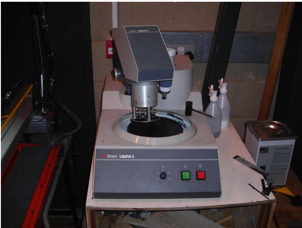
Figure 24: STRUERS LaboPol-5 polishing machine
