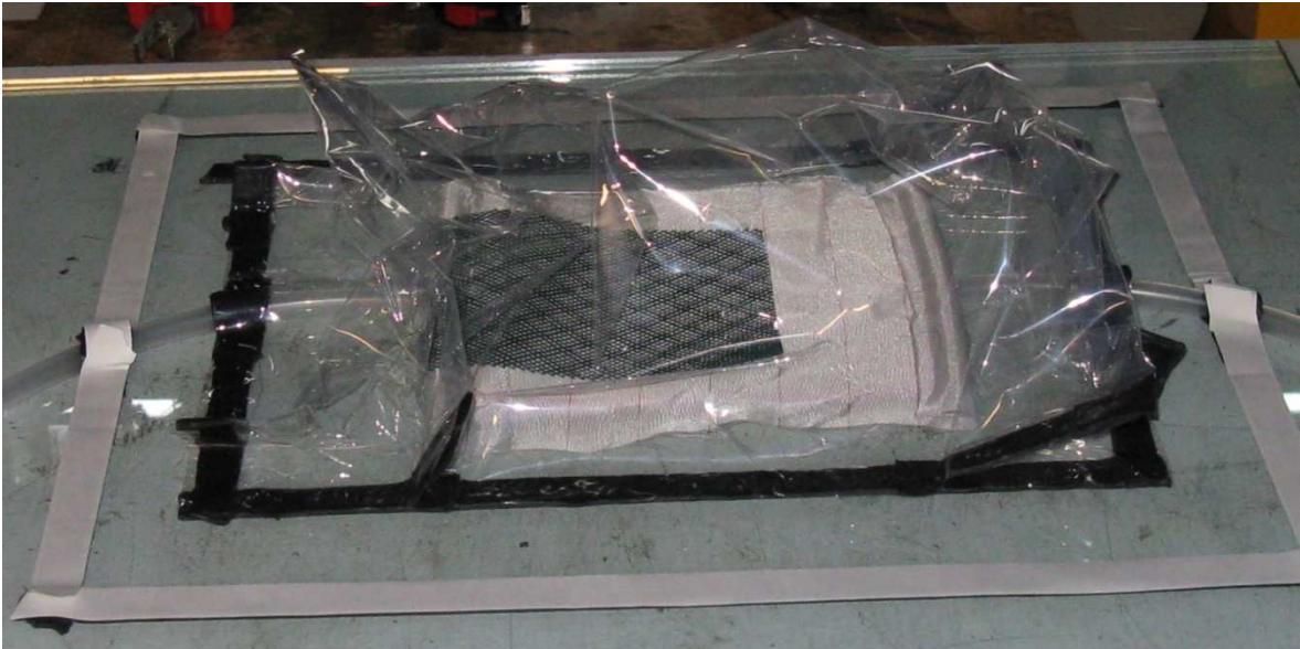
Figure 21: Mould with Vacuum Bag
