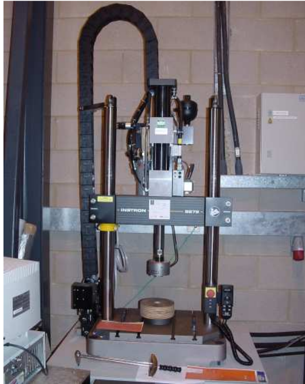
Figure 43: INSTRON 8872 Fatigue Testing Machine
