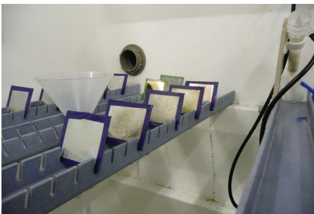
Figure 4-8: Digital Image showing a typical sample configuration for an NSS test.
