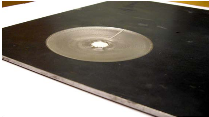
Figure 2. Circular indentation of power-law profile materialising a two-dimensional acoustic black hole for flexural waves in plates.
