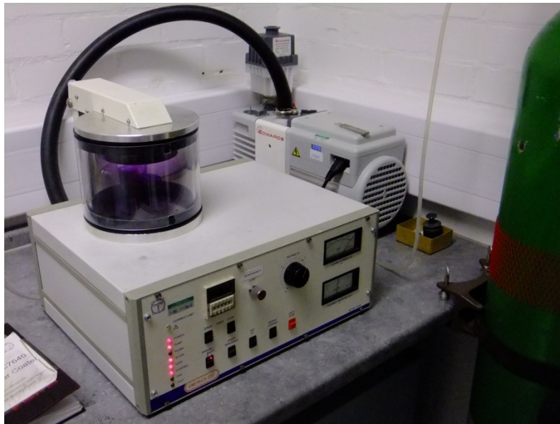
Figure 9-4: EMTECH Au-Pd sputter coater coating sample
