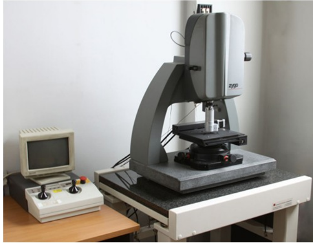
Figure 5-2: Zygo interferometer and its control equipment
