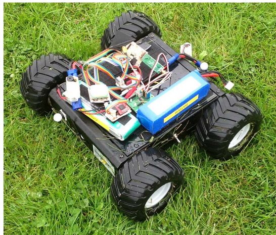
Figure 7.14: Lynxmotion Rover with Avionics Fitted
