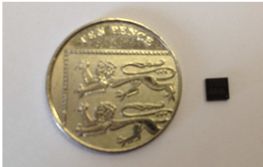
Figure 2.14: Automotive Grade MEMS Sensors Used in this Thesis
