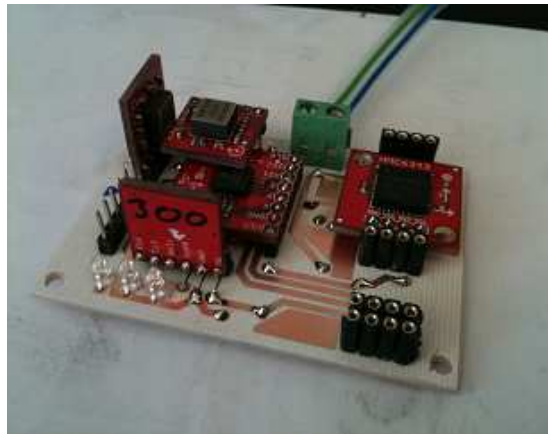
Figure 7.7: Low Cost MEMS Sensors Used for AHRS
