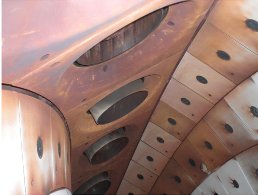
Figure 5.16 A photograph taken from within the engine combustion chamber showing the modified burner rings; this is the location directly opposite the five test tiles.
