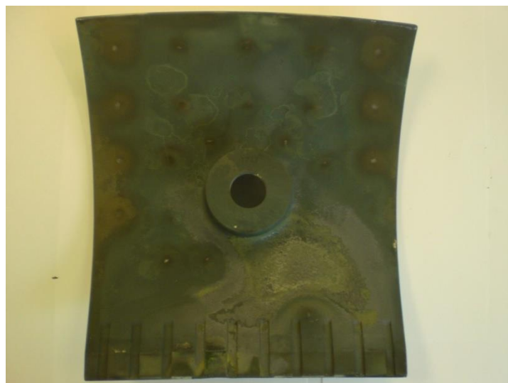
Figure 5.17 A photograph showing the underside of the tile and the updated tile design with additional cooling slots to try and prevent tile overheating.
