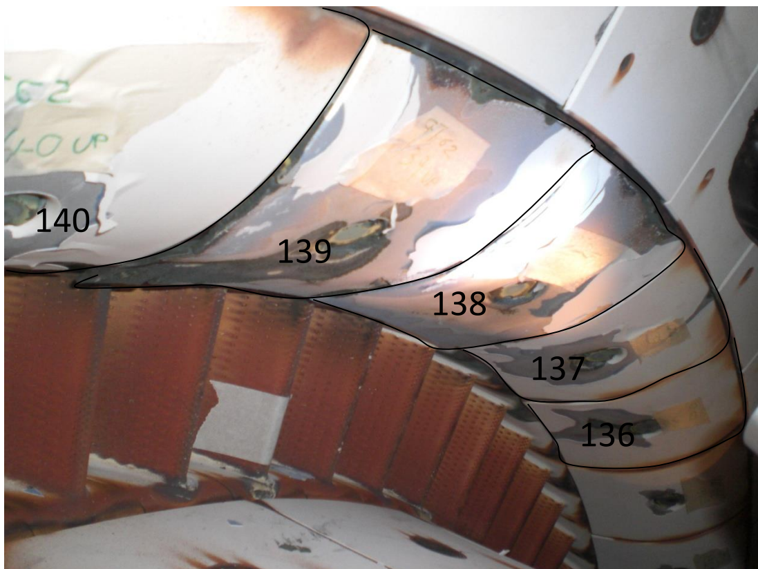
Figure 5.15 A photograph taken from within the engine combustion chamber showing the tiles in their specific locations. The five tiles characterised within this piece of work are highlighted, numbered 136, 137, 138, 139 and 140.
