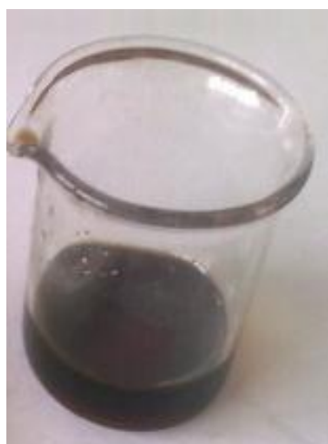
Figure 9F.1 – Effect of long-term heat treatment on butyltrimethylammonium bis(trifluoromethylsulfonyl)imide liquid after 18 hours heating at 250 °C in air.
