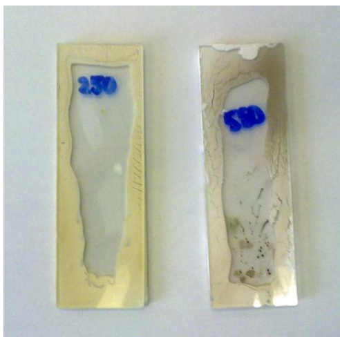
Figure 9.12 – Heat test of glass frit (flux 23901, Johnson-Matthey) after one hour at 250 °C (left) and one hour at 550 °C (right).
