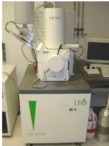
Figure 2.17 – The FEG-SEM instrumentation used in this thesis. Model: Carl Zeiss (Leo) 1530 VP.
