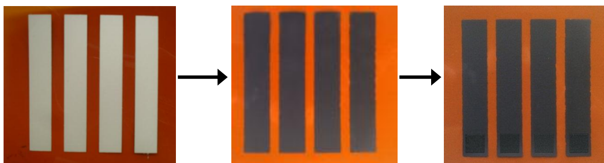
Figure 9.15 – Photographs of screen printed electrodes. Silver conducting layer (left), smooth carbon intermediate layer (middle), and activated carbon layer (right).
