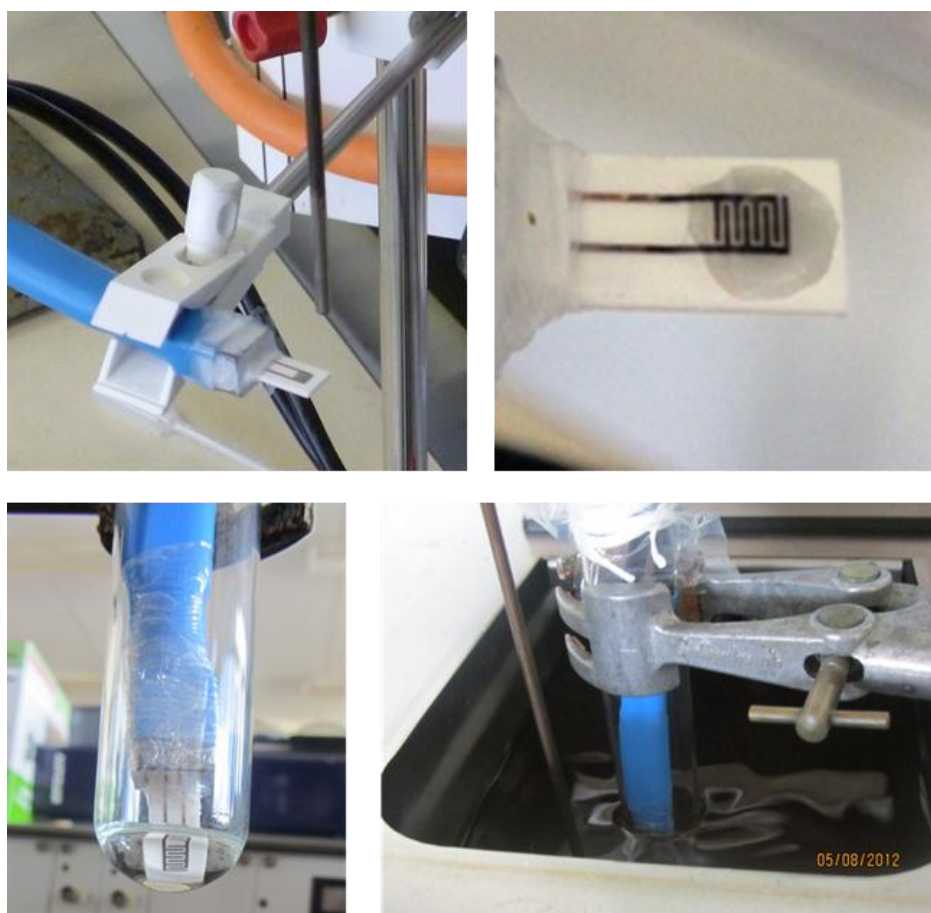
Figure 7.21 – A photograph illustrating the set-up for measuring the conductivity of an ionic liquid in a single droplet (top) and a small sample volume (bottom) using a PIG electrode.
