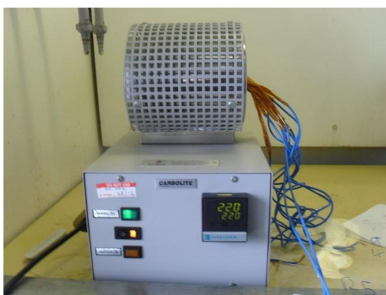
Figure 9.23 – The tube furnace used for testing the long term stability of screen printed supercapacitors.
