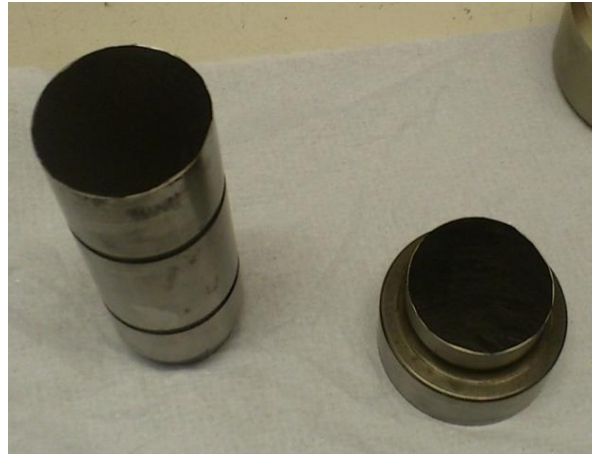
Figure 3.3 Teflon sheets attached on the \varnothing 40 mm die surfaces to prevent the powder sticking.
