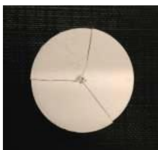
Figure 6.33 A broken sample after impact test.
