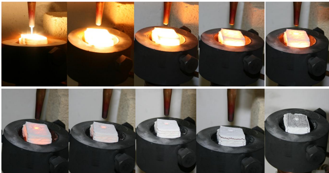
Figure 4.60: Series of images taken during and immediately after oxyacetylene testing showing spallation of the oxide layer for Cf-HfC composite
